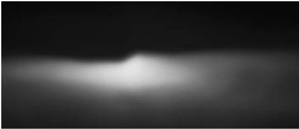
Figure 2 Photograph of a low beam headlight pattern projected onto a vertical surface (5); the horizontal cutoff on the right side of the image corresponds to a vertical angle of 0°
