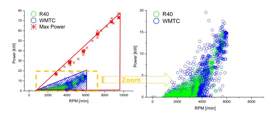
Larger area covered by WMTC → maximized sampling in the part-load area
