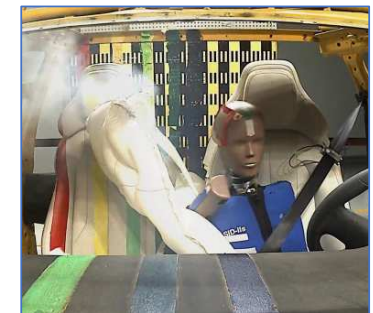
SID2S arm is located on the side of the airbag
