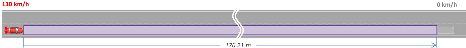
$$s_{front} = \frac{(v_{S, max})^2}{2 * a_{VUT}}$$
