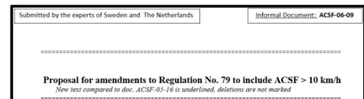
This proposal describes the necessity to detect objects, pedestrian and animals. The distance that such kinds of “things” have to be detected to start a protective/emergency braking should be defined to 60m.
