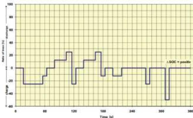
Figure 106. ISO 12405-2 Profile for cycle life test — Plug-in charge-rich current profile [102]
