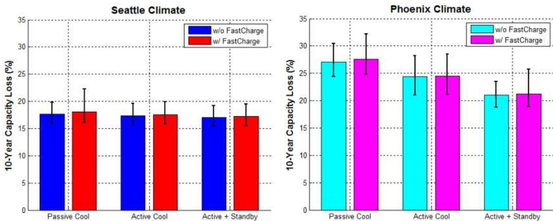
Figure 41. Effect of DCFCs and BTMS on battery capacity loss in Seattle (left) and Phoenix (right) [66]
