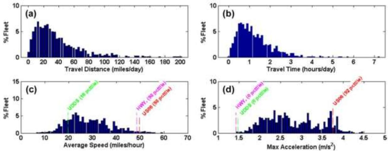
Figure 53. Drive-cycle metrics (a) distance-traveled per day, (b) travel time per day, (c) average speed while driving, and (d) maximum acceleration. Blue histograms represent 782 drive-cycles from Texas survey [69].
