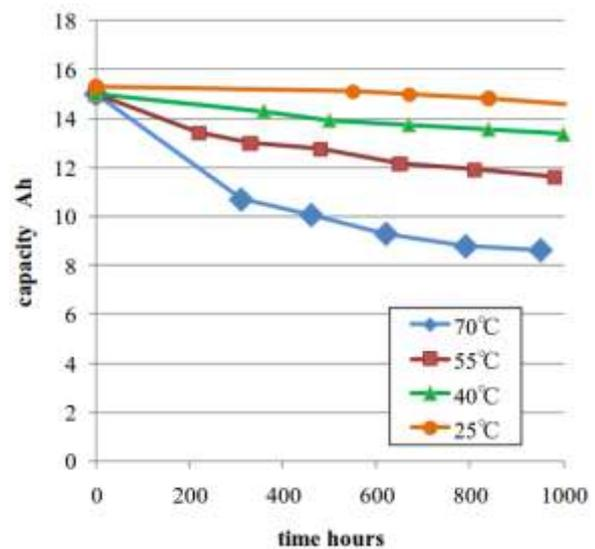
Figure 89. decrease of Ah capacity in each of the temperature conditions [86]
