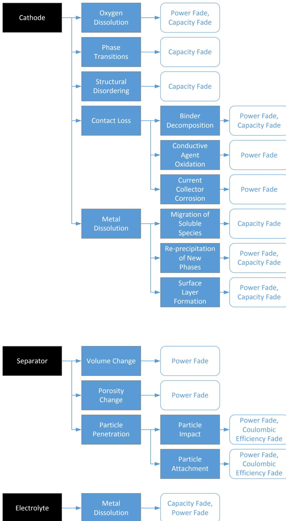
Figure A 2 Degradation Mechanisms of the Cathode, Separator, and Electrolyte [46]
