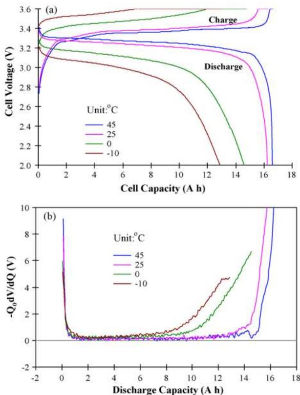
Figure 73. (a) Charge–discharge curves at 1C rate measured at different temperatures for a fresh cell and (b) the corresponding differential voltage ( $-Q_0 dV/dQ$ ) versus discharge capacity. [81]
