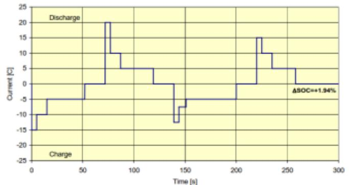
Figure 103. ISO 12405-1 — Current profile for cycle life test — Charge-rich profile [101]
