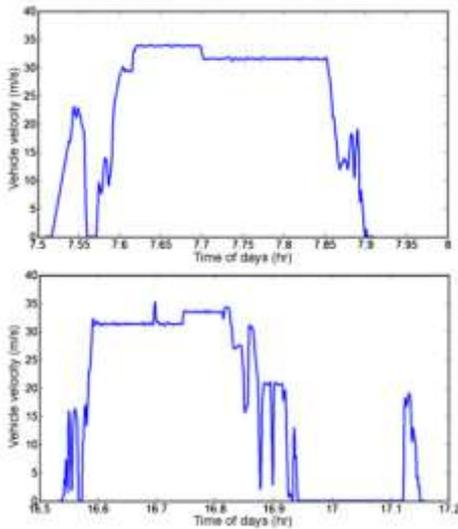
Figure 36. A sample suburban naturalistic drive cycle with two half trips, one in the morning and one in the afternoon (vehicle velocity is zero during the rest of the day) [63]
