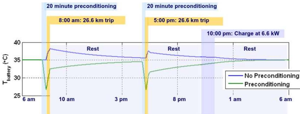
Figure 62. Battery temperature and SOC profiles for PHEV40s @ 35°C ambient temperature, with/without thermal preconditioning [72]
