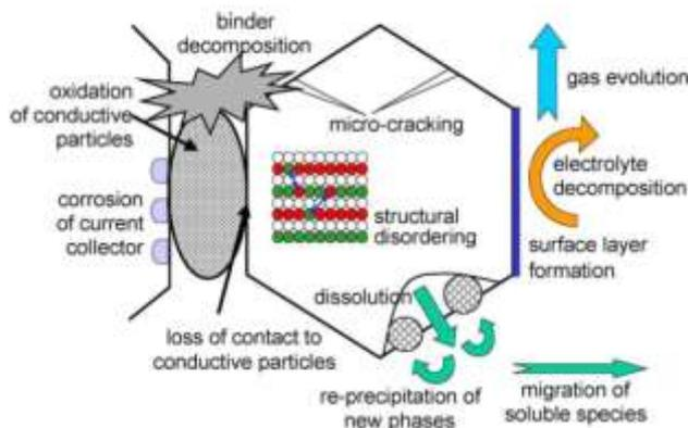
Figure 11. Degradation mechanisms for the positive electrode [28]
