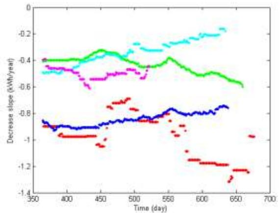
Figure 48. Average battery capacity evolution with a two-year sliding window centered with day mentioned on X-axis (red: EV1; green: EV2; blue: EV3; cyan: EV4; magenta: EV5) [68]
