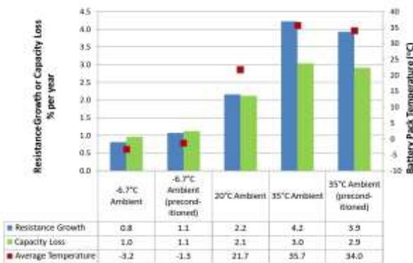
Figure 60. PHEV40s battery degradation rates (left axis) and average temperature (right axis) [72]
