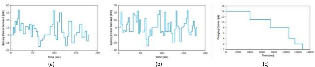
Figure 79. Degradation test procedure profiles for (a) PHEV CD test, (b) PHEV CS test, and (c) PHEV charging profile [83]
