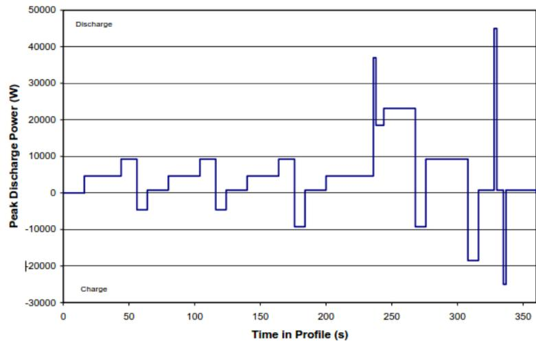
Figure 97. Charge-Depleting PHEV-20 Mile Battery Cycle Life Test Profile [82]
