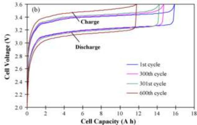
Figure 72. Cycling performance at 3C rate between 3.6 and 2.0 V at 50°C: charge–discharge loops for the beginning and last cycles of the 1st 300 cycles (1st and 300th cycles) and the 2nd 300 cycles (301<sup>st</sup> and 600<sup>th</sup> cycles). [81]
