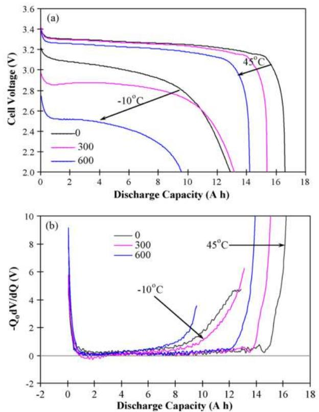
Figure 74. (a) Discharge curves at 1C rate measured at 45 and  $-10^{\circ}\text{C}$  after different cycles and (b) the corresponding differential voltage ( $-Q_0 dV/dQ$ ) with respect to discharge capacity. [81]
