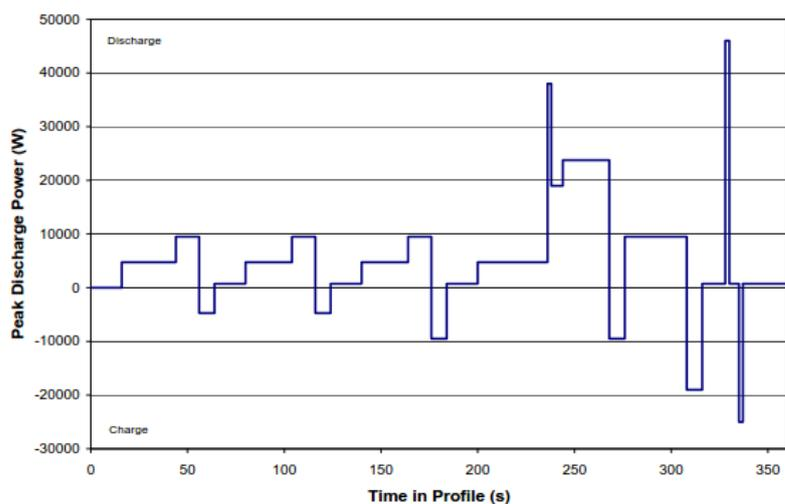
Figure 98. Charge-Depleting PHEV-40 Mile Battery Cycle Life Test Profile [82]
