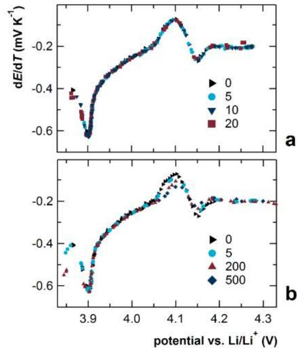
Figure 22. Thermodynamic data for  $\text{LiCoO}_2$  from Figure 19 and Figure 21 expressed as  $dE/dT$  vs. OCP (entropy vs. Gibbs free energy). The  $\text{LiCoO}_2$  electrodes were cycled at (a) the “fast” rate of  $C/2$  and (b) the “slow” rate of  $C/5$ , and the number of cycles is shown in the legends. All of the data points from three identically prepared cells for each condition (cycling rate and number of cycles) are shown individually [47].
