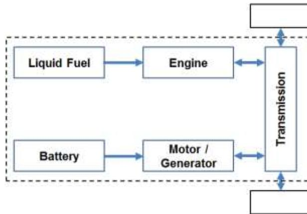
Figure 5. Basic Architecture of a Parallel HEV
