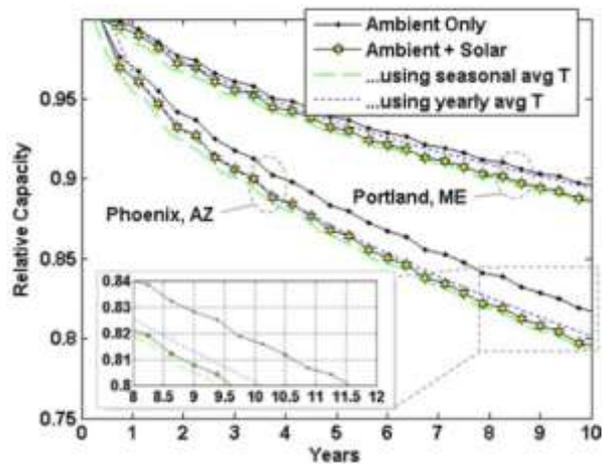
Figure 56. Capacity fade under storage at 90% SOC for two geographic locations with and without impact of solar loading on the parked vehicle [69]
