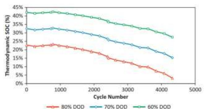
Figure 83. Thermodynamic SOC relative to capacity based DOD as a function of cycle number [83]
