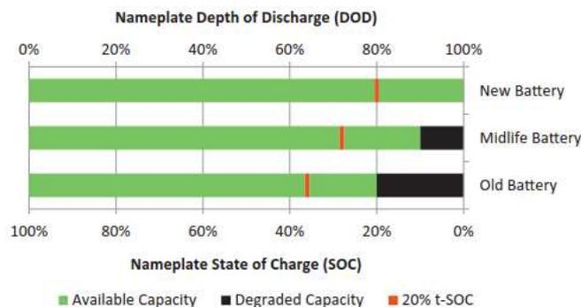
Figure 78. Variation of t-SOC as a result of capacity degradation. As the battery degrades, the degraded capacity occupies a greater fraction of nameplate SOC, whereas t-SOC is normalized to the available capacity. [83]
