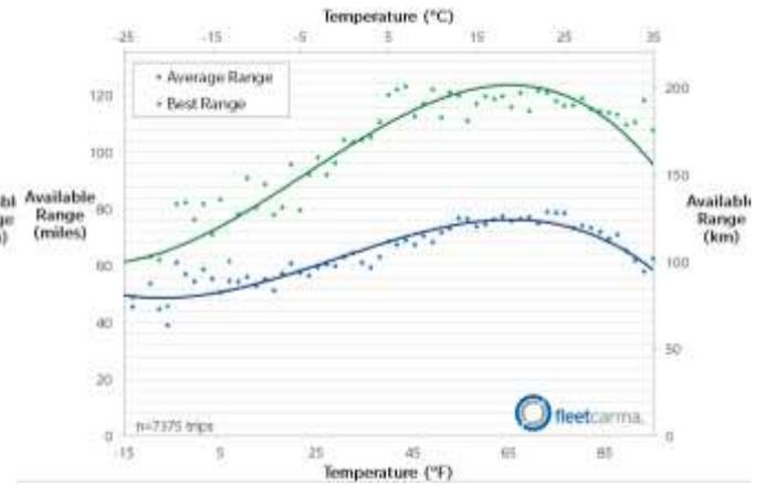
Figure 67. Nissan Leaf: Range vs. Temperature spanning all model years in the FleetCarma database [77]
