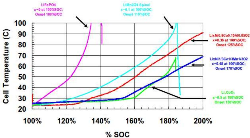
Figure 25. Heat output during overcharge for different cathode oxide chemistries, showing an increase in heat output when final lithium is removed from the cathode. [52]
