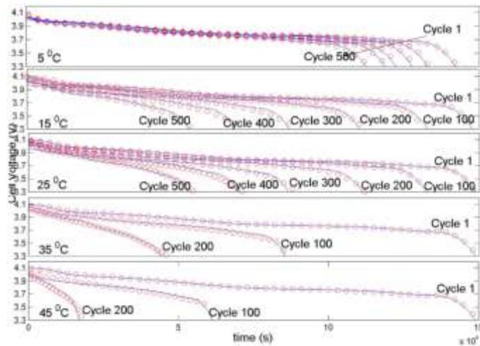
Figure 69. Degradation of cell voltage for increasing cycles at various temperatures [78]
