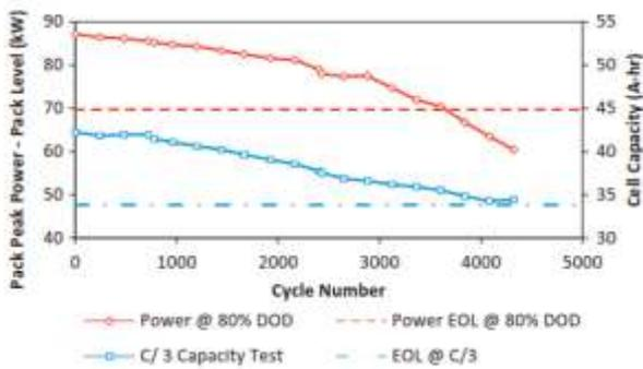
Figure 80. Energy and power measurements as a function of cycle number (fig5) [83]
