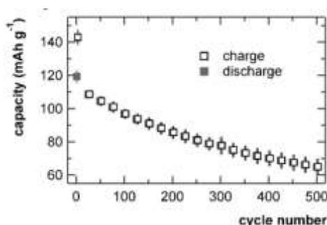
Figure 20 Specific (gravimetric) capacity of galvanostatically cycled cells containing LiCoO<sub>2</sub> cathodes and MCMB anodes. Cycling rate was C/10 (charge) and C/5 (discharge) for the first five cycles and C/5 (charge and discharge) thereafter. Markers and error bars are the average and standard deviation, respectively, of measurements from three identically prepared cells.
