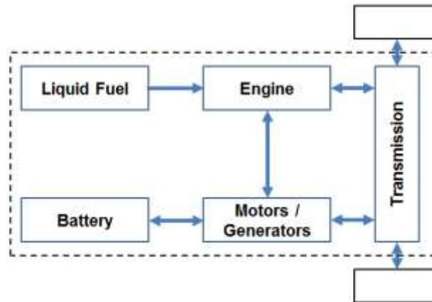
Figure 3. Basic Architecture of a Series-Parallel HEV
