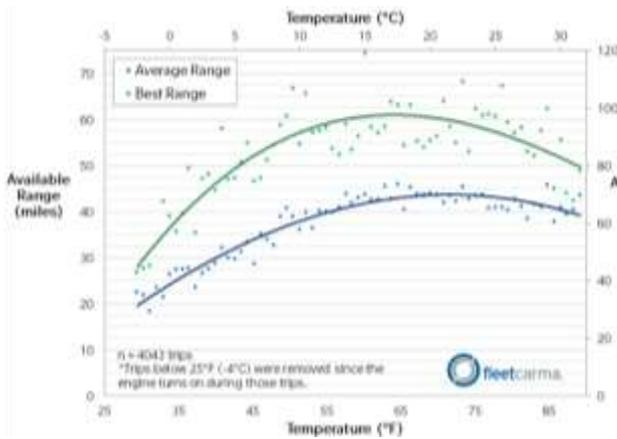
Figure 66. Chevrolet Volt: Electric Range vs. Temperature spanning all model years in the FleetCarma database [77]
