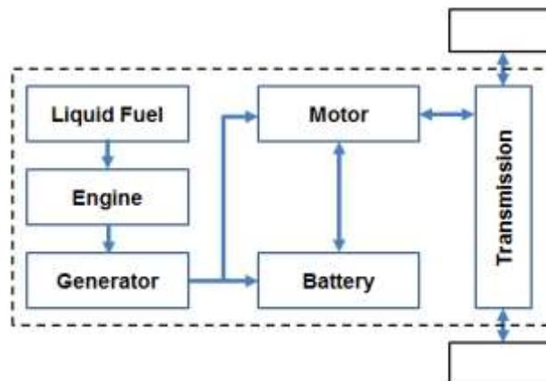
Figure 4. Basic Architecture of a Series HEV
