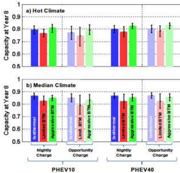
Figure 64. Remaining capacity at the end of 8 years for various BTM and charging scenarios. Colored bars show average result for all 782 drive cycles. Error bars show result for 5<sup>th</sup> and 95<sup>th</sup> percentile drive cycles. [75]
