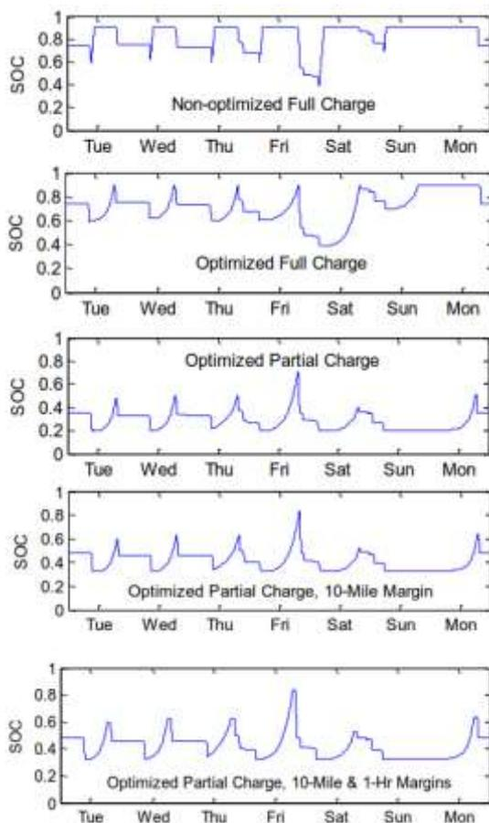
Figure 38. Weekly SOC profiles for the four charging methods. Horizontal axis labels indicate the beginning (midnight) of each day. [64]
