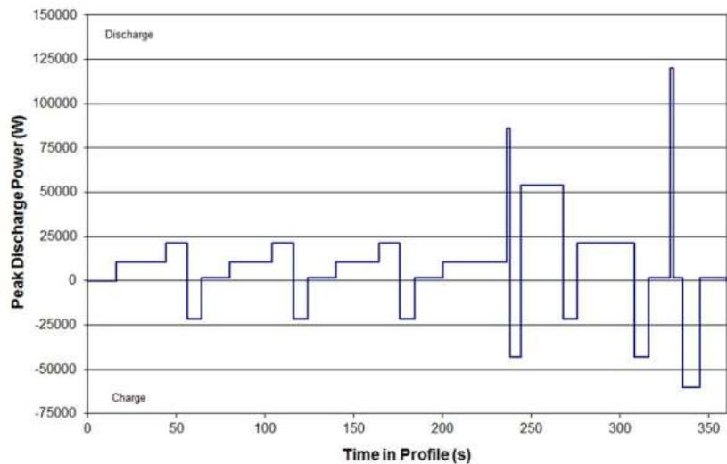
Figure 99. Charge-Depleting Cycle Life Test Profile for the xEV-50 Mile Battery [82]
