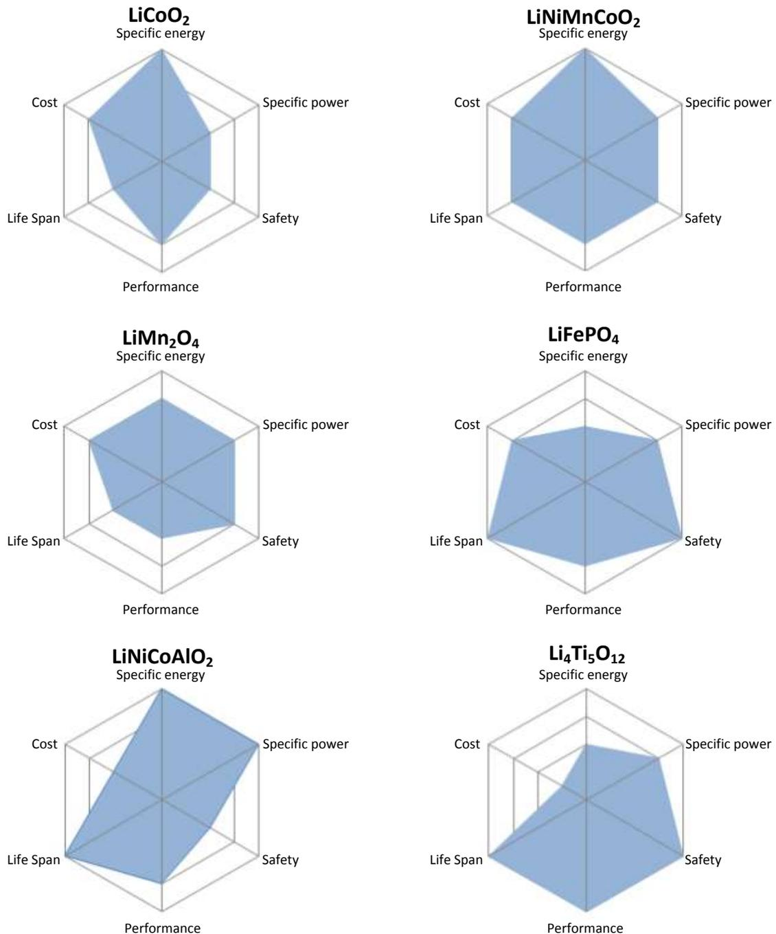
Figure 7. Properties of different Li-ion cell chemistries [7]
