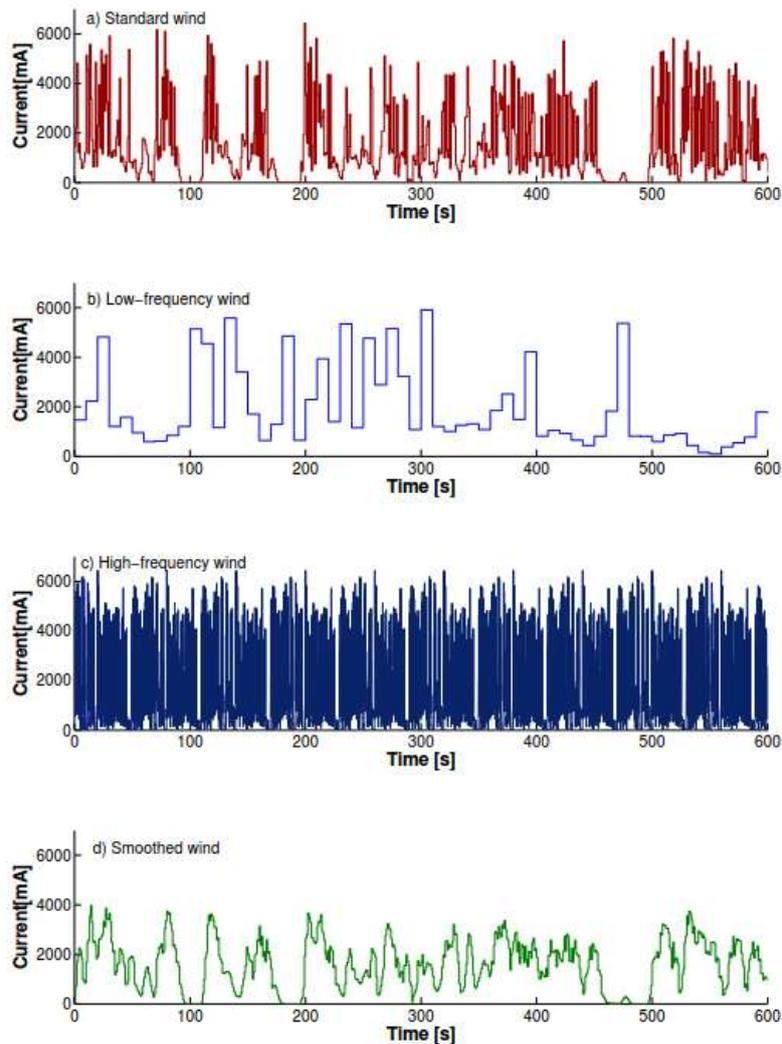
Figure 42. 600s data series of the a) standard wind, b) low-frequency wind, c) high-frequency wind, and d) smoothed wind current profiles, derived from the output current of a 150W wind turbine [29].
