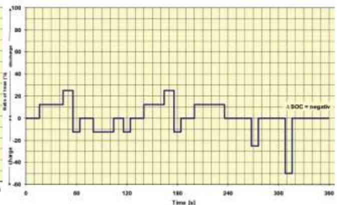
Figure 107. ISO 12405-2 Profile for cycle life test — Plug-in discharge-rich current profile [102]
