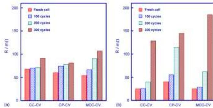
Figure 46. Comparison of the ohmic resistance (a) and charge-transfer resistance (b) for 18650 cells by different charging protocols. [67]
