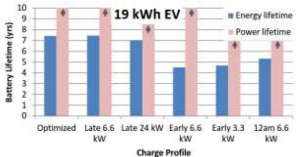
Figure 86. 19 kWh battery lifetime under various charge scenarios. Power lifetimes truncated.
