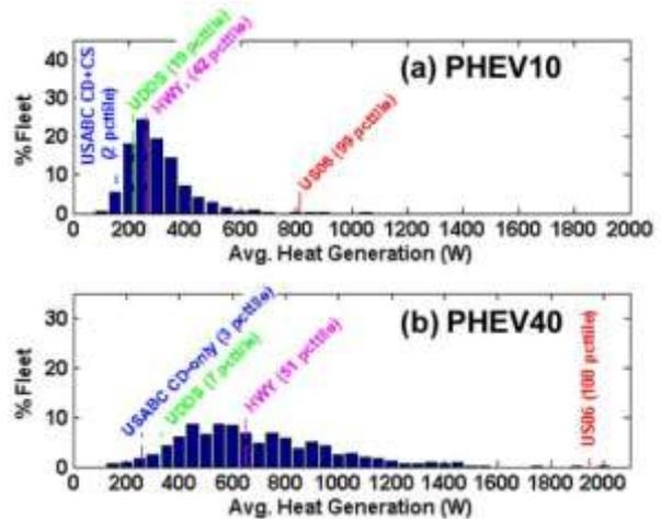
Figure 55. Model-predicted average heat generation rate during driving [69]
