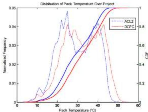
Figure 50. Battery pack temperature distribution for ACL2 and DCFC vehicles. The data represents 50,000 miles of driving, charging, and parking over more than 500 days [62]
