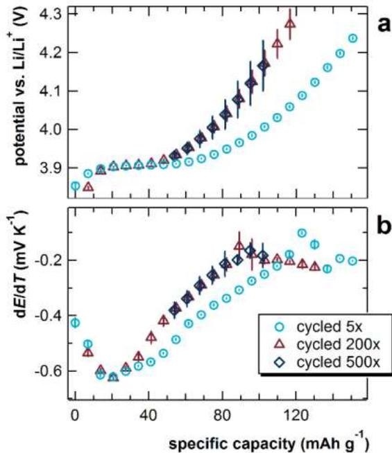
Figure 21. (a) Open-circuit potential and (b)  $dE/dT$  of half-cells containing  $\text{LiCoO}_2$  cathodes and lithium anodes. The  $\text{LiCoO}_2$  electrodes were cycled in full cells (vs. MCMB) according to the conditions in Figure 20 ( $C/5$  rate), removed from the full cells, and then placed in new half-cells for the measurements in a and b. Markers and error bars are the average and standard deviation, respectively, of measurements from three identically prepared cells [47].
