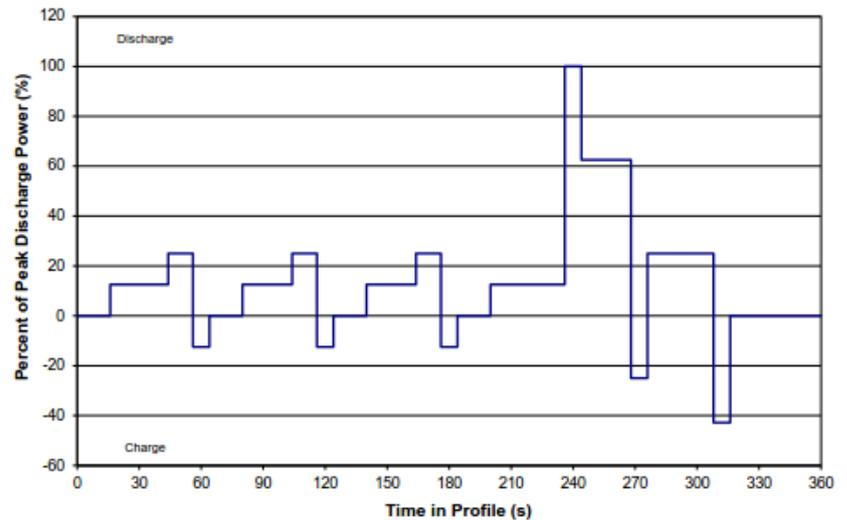
Figure 100. Charge-Depleting Cycle Life Test Profile for the BEV Battery [84]
