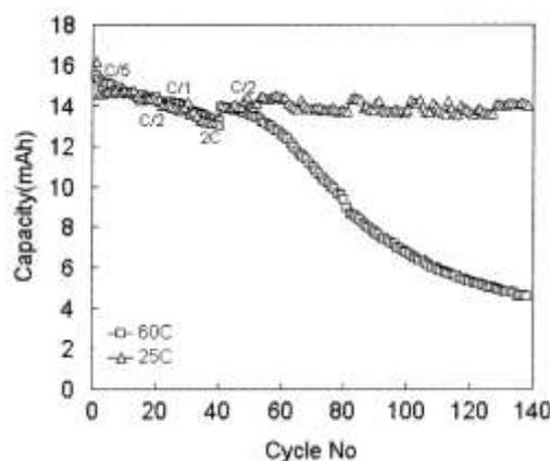
Figure 24. Cycling performance for pouch cells at 25 and  $60^\circ\text{C}$ . Cut-off voltage 3.0-4.1V [48]
