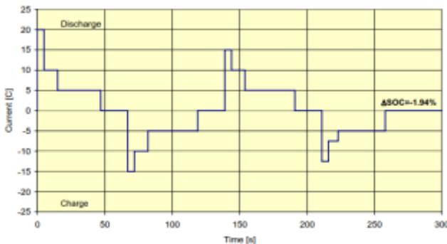
Figure 102. ISO 12405-1 — Current profile for cycle life test — Discharge-rich profile [101]
