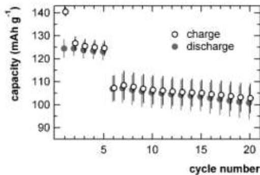
Figure 18. Specific (gravimetric) capacity of galvanostatically cycled half-cells containing  $\text{LiCoO}_2$  cathodes and lithium anodes. Cycling rate was  $C/5$  (charge) and  $C/2$  (discharge) for the first five cycles and  $C/2$  (charge and discharge) thereafter. [47]
