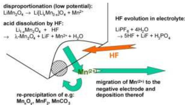
Figure 12. Dissolution of lithium manganese spinel [18]
