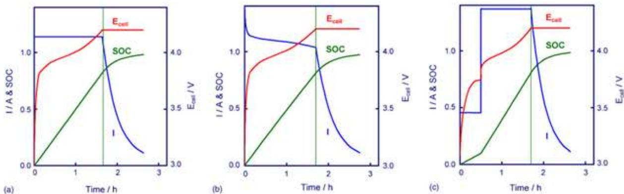
Figure 45. Characteristics of the charging protocols for a commercial 2.4Ah 18650 Li-ion cell using an averaged charging rate of 0.5C
