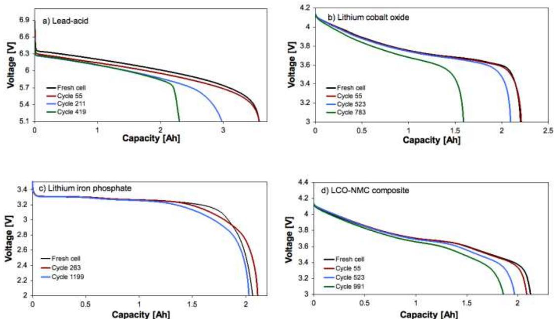
Figure 44. Discharge voltage curves after capacity tests in wind-aged a) lead-acid, b) LCO c) LFP and d) medium-frequency wind-charged LCO-NMC cells (Figure 4.2 from source) [29].
