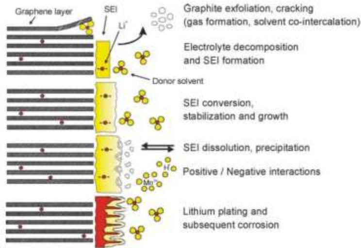
Figure 10. Degradation Methods for the Negative Electrode [18]
