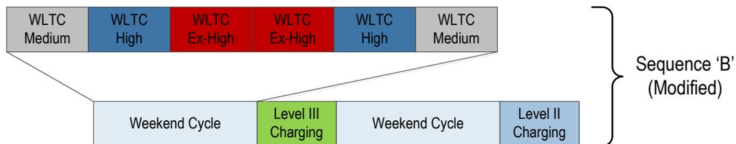
Figure 111. Modified sequence showing two charging methodologies in use
