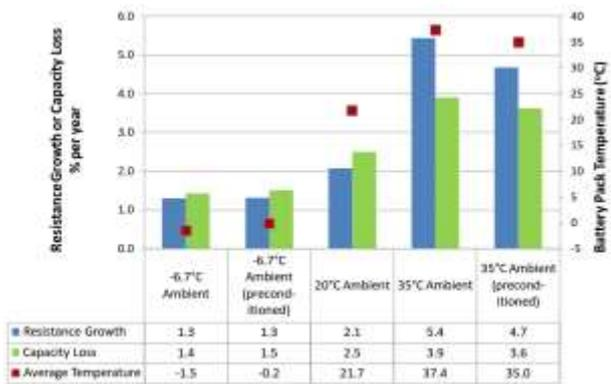
Figure 61. EV battery degradation rates (left axis) and average temperature (right axis) [72]
