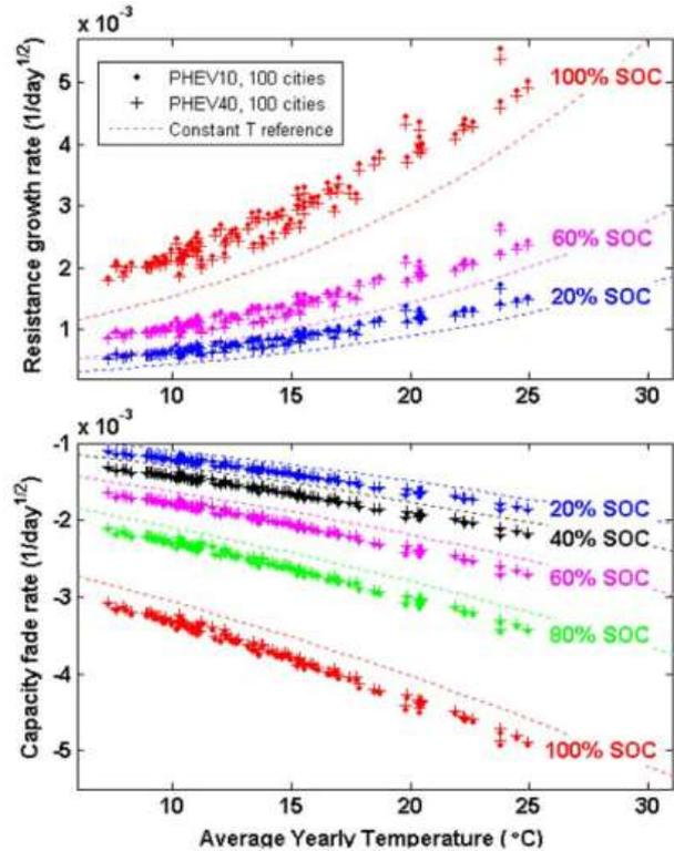
Figure 52. Resistance growth and capacity fade rates under storage at constant SOC. Reference lines show results for constant temperature. Symbols show simulated results for PHEVs using hour-by-hour TMY ambient temperature and solar radiation data for 100 U.S. cities [69]
