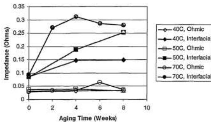
Figure 16. Changes in Interfacial Impedance and Ohmic Resistance after Aging at Different Times and Temperatures. [45]
