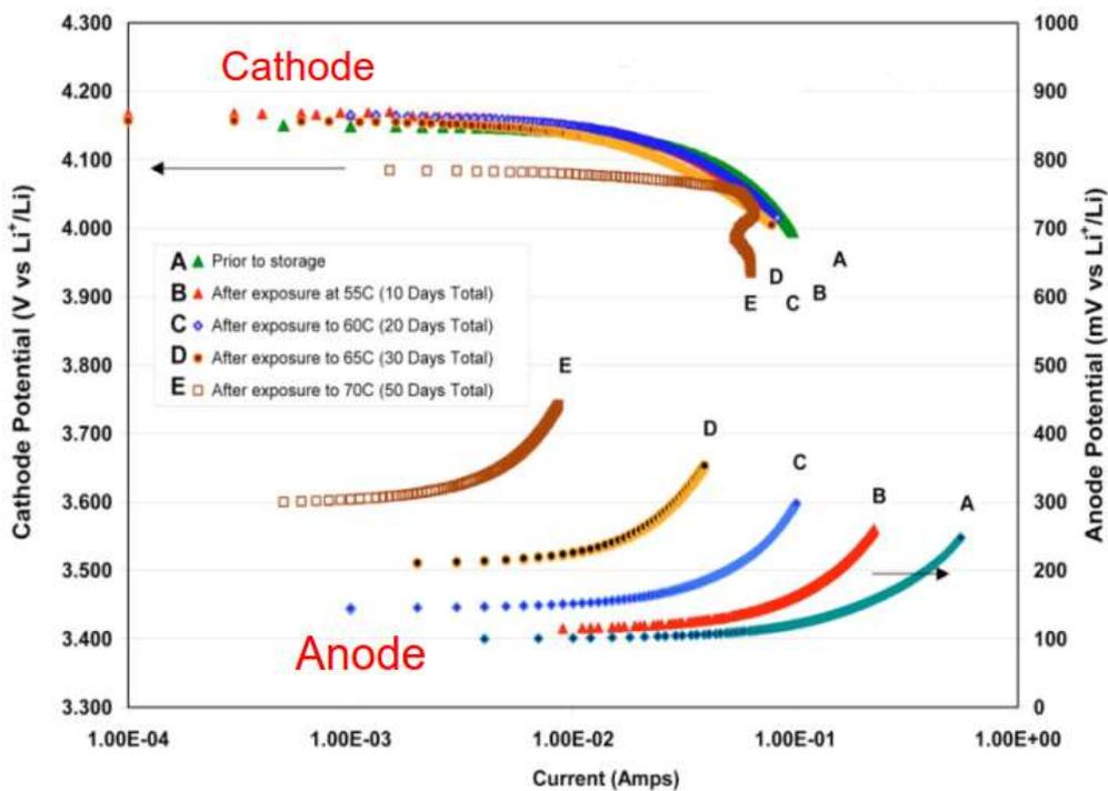
Figure 65. Half-cell Potentials from cells subjected to aging at different temperatures: Side reactions happen faster on the electrode surface with increase in the temperature – resulting in faster build-up of the resistance at the electrode surface [76]
