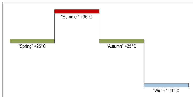
Figure 112. Simulated Year Cycle Climate for Durability Testing
