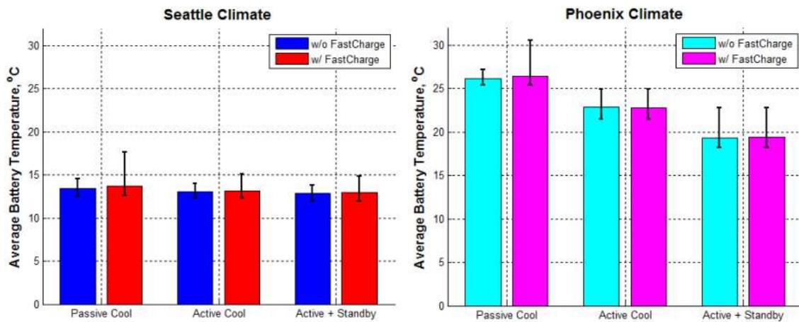
Figure 40. Effect of DCFCs and BTMS on average battery temperature in Seattle (left) and Phoenix (right) [66]
