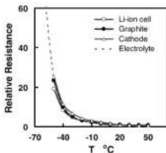
Figure 14. Li-Ion Battery Resistance Increases with Decreasing Temperature [39]
