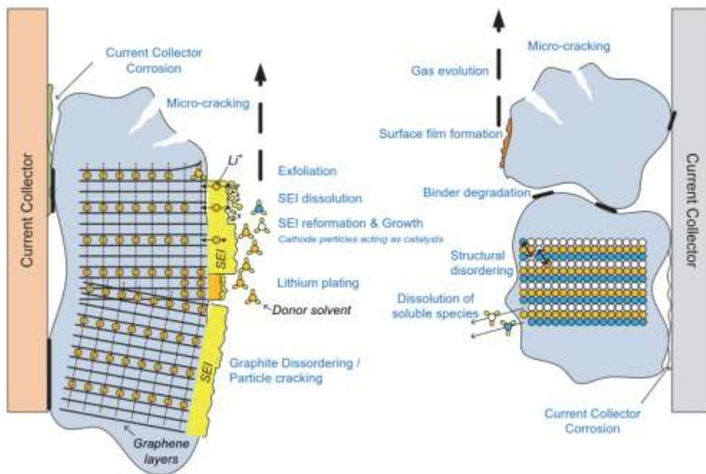
Figure 30. Aging mechanisms occurring at Li-ion battery electrodes [58]
