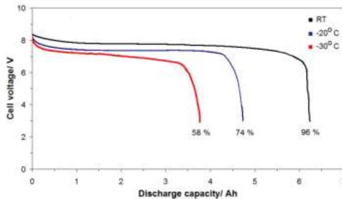
Figure 29. Discharge curves for a 6.5Ah NiMH prismatic battery module, recorded for a discharge rate of 0.15C at: room temperature (RT), -20, and -30°C [57]
