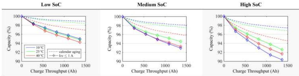
Figure 70 Comparison of calendar aging and cyclic aging for the three temperatures investigated [79]
