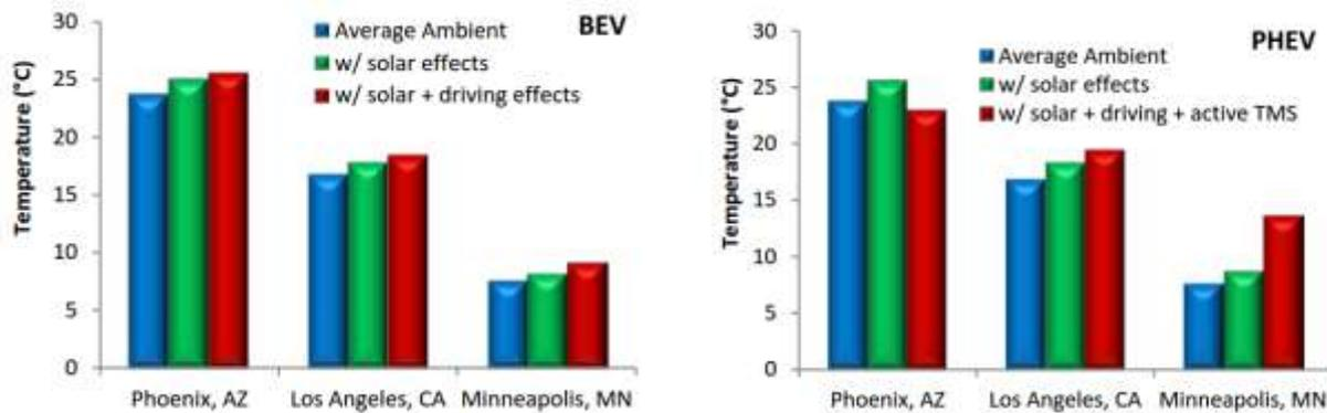
Figure 71. Average yearly battery temperature contributions from ambient, solar loading, and internal heat generation for simulated (a) BEV and (b) PHEV. [80]
