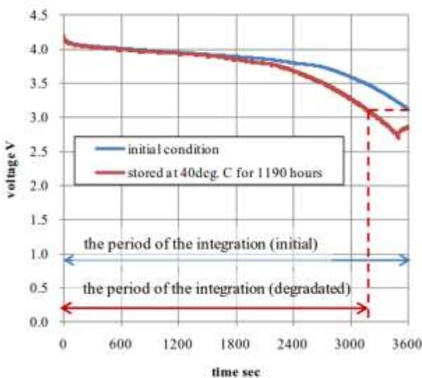
Figure 88. Comparison of the discharge characteristics of a battery which was initially not stored at 40°C at beginning of testing and after 1190 hours of storage at 40°C [86].
