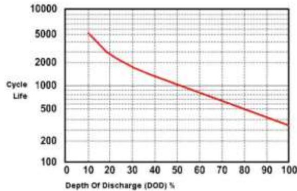
Figure 28. Example of the dependence of cycle life on DOD in a NiMH battery [54]
