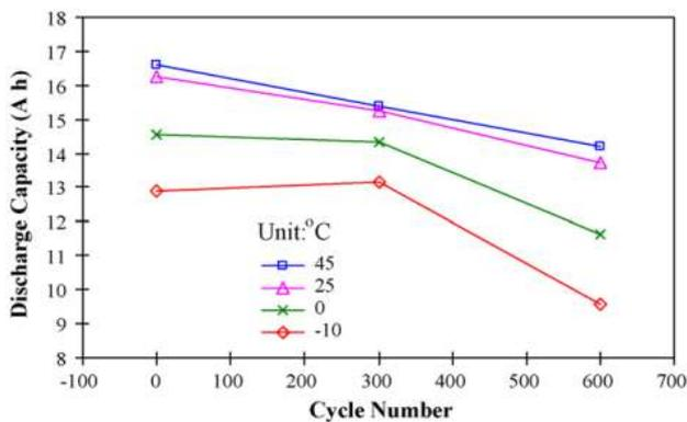
Figure 75. Discharge capacity measured at different temperatures varying with cycle number.
