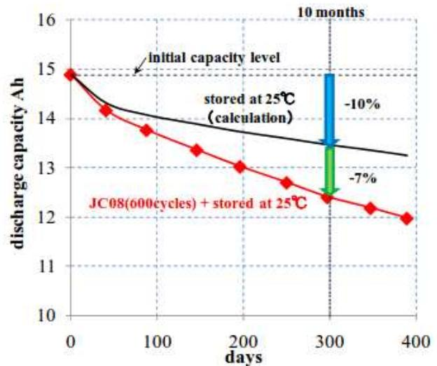
Figure 91. Variation of the discharge capacity against time in days [86]
