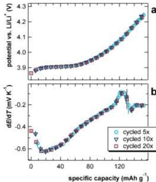
Figure 19. (a) Open-circuit potential and (b)  $dE/dT$  of half-cells containing  $\text{LiCoO}_2$  cathodes and lithium anodes after cycling according to the conditions in Figure 18 ( $C/2$  rate). [47]
