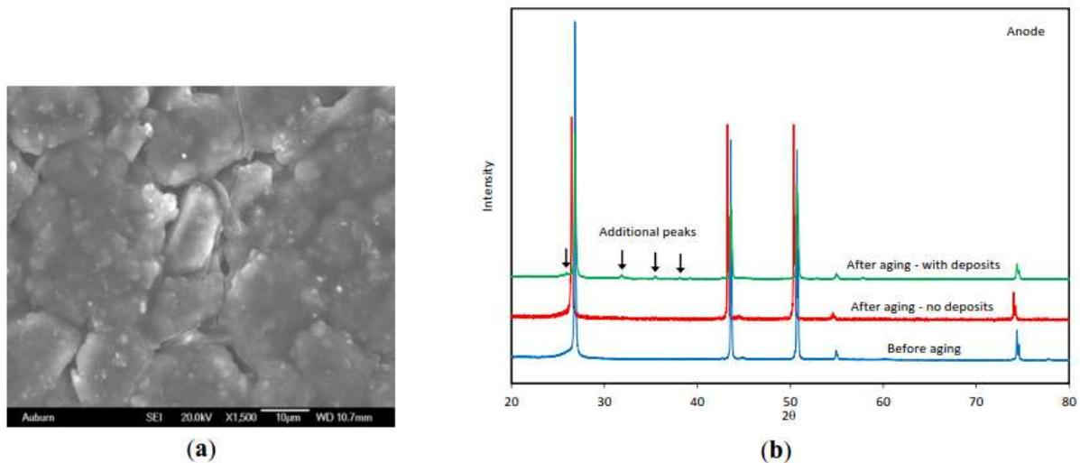
Figure 9. Structural changes on the anode electrode from degradation. (a) Surface cracks on the surface of aged anode electrode; (b) XRD spectra of aged anode electrode showing change in crystal structure (new phases). [19]
