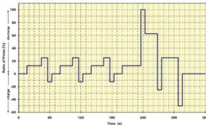
Figure 104. ISO 12405-2 Profile for cycle life test — Dynamic discharge power profile A [102]
