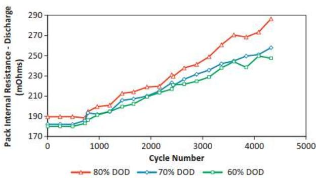
Figure 82. Pack internal discharge resistance as a function of cycle number [83]
