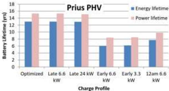
Figure 85. Prius battery lifetime under various charge scenarios
