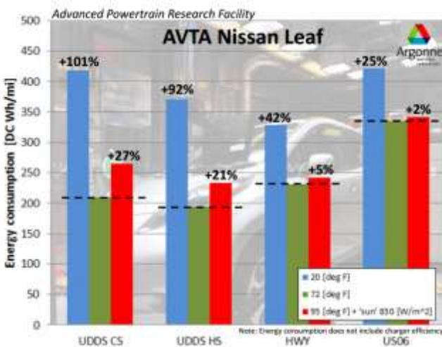
Figure 57. Impact of Temperature on Energy Consumption [70]
