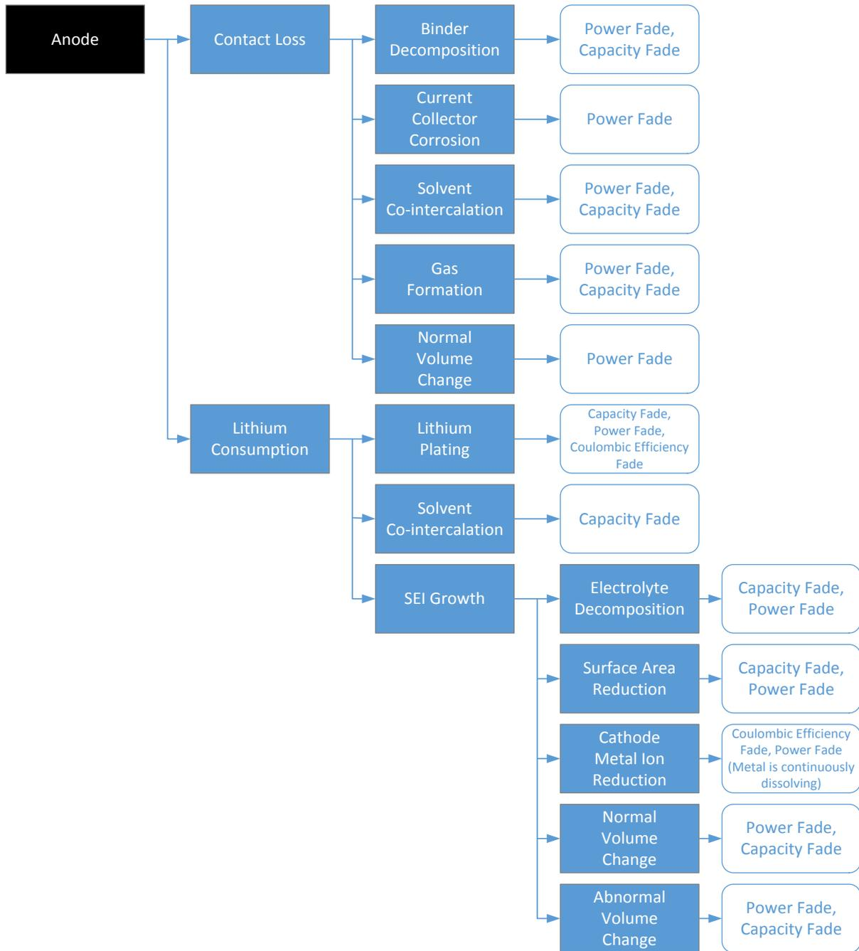
Figure A 1 Degradation Mechanisms of the Anode [46]
