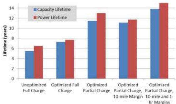
Figure 39. Comparison of battery energy and power lifetimes under the five charging scenarios. One power lifetime result over 15 years is truncated. [64]
