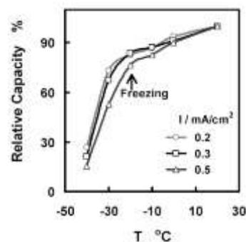
Figure 15. Li-Ion Battery Capacity Decreases with Decreasing Temperature [39]
