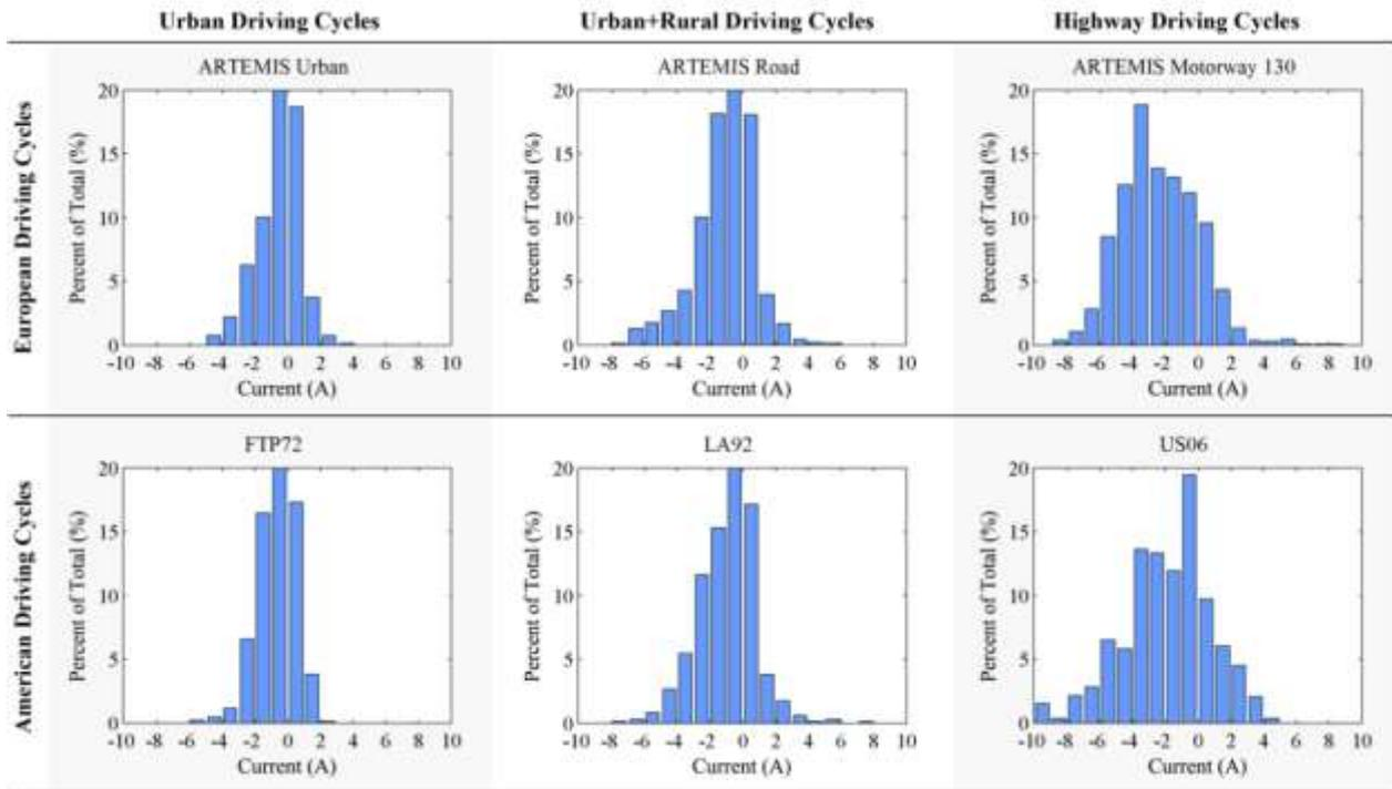
Figure 93. Distribution of cell currents for different European and American driving cycles as percent of total driving cycle duration [79]
