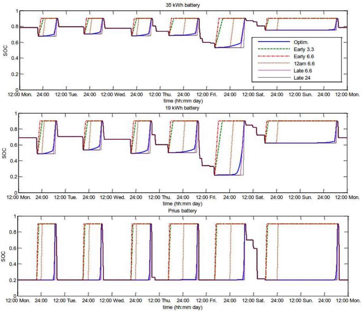
Figure 84. Weekly SOC profiles for three battery sizes under various charging scenarios
