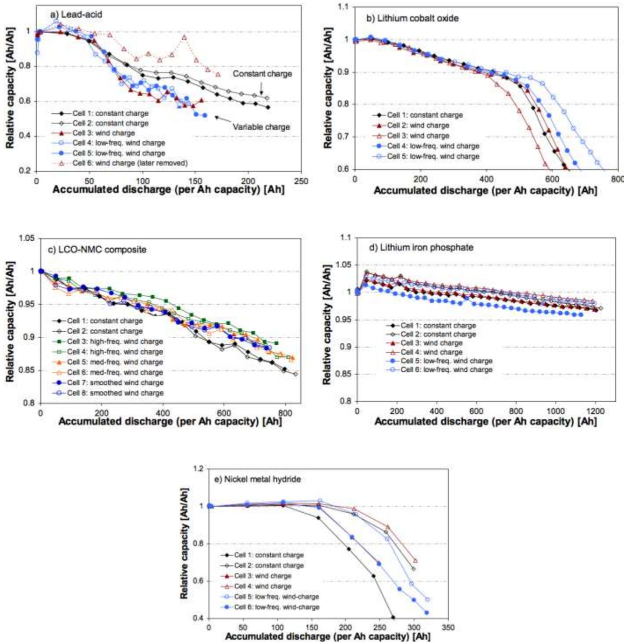
Figure 43. Capacity fade as a function of normalized discharge throughput in a) lead-acid, b) LCO c) LCO-NMC d) LFP cells and e) NiMH cells. [29]
