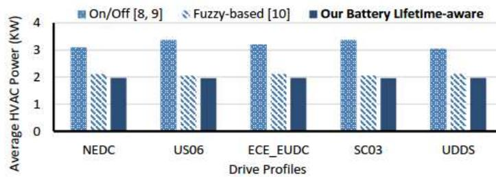
Figure 63. HVAC Power Consumption Analysis for Different Drive Profiles [73]
