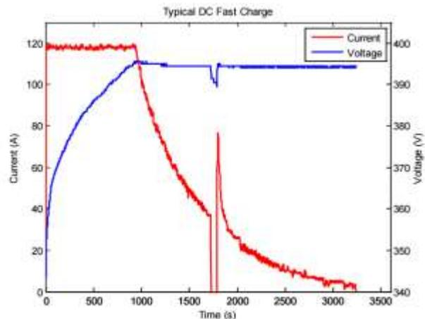
Figure 32. A DC fast charge is shown for a 2012 Nissan Leaf charged with a 50kW fast charger. The charge automatically ended after 1725 seconds, and another charge session was initiated shortly after the first one ended to fully charge the battery [62]
