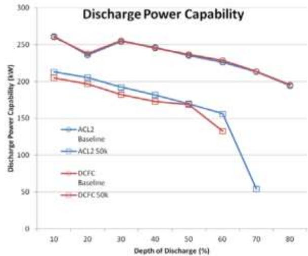
Figure 34. Average discharge power capability versus depth of discharge for ACL2 and DCFC groups at baseline and after 50,000 miles. [62]
