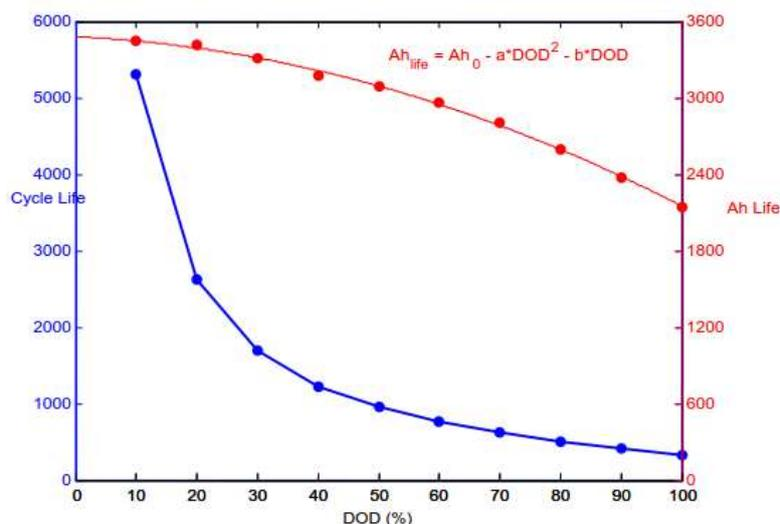
Figure 27. Comparison of cycle life and Ah life (the scale of Ah life is not accurate because it is based on an arbitrary value of nominal capacity. However the shape of the curve is independent from that value). [54]
