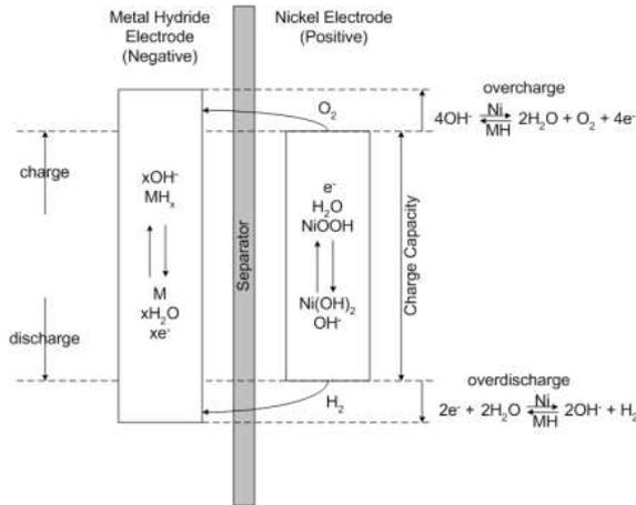
Figure 26. Schematic Representation of NiMH Cell
