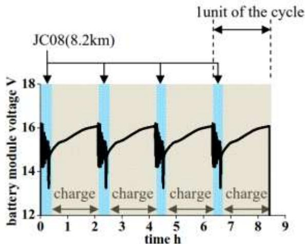
Figure 90. Voltage variation of the test battery module with the JC08 charge/discharge patterns [86]
