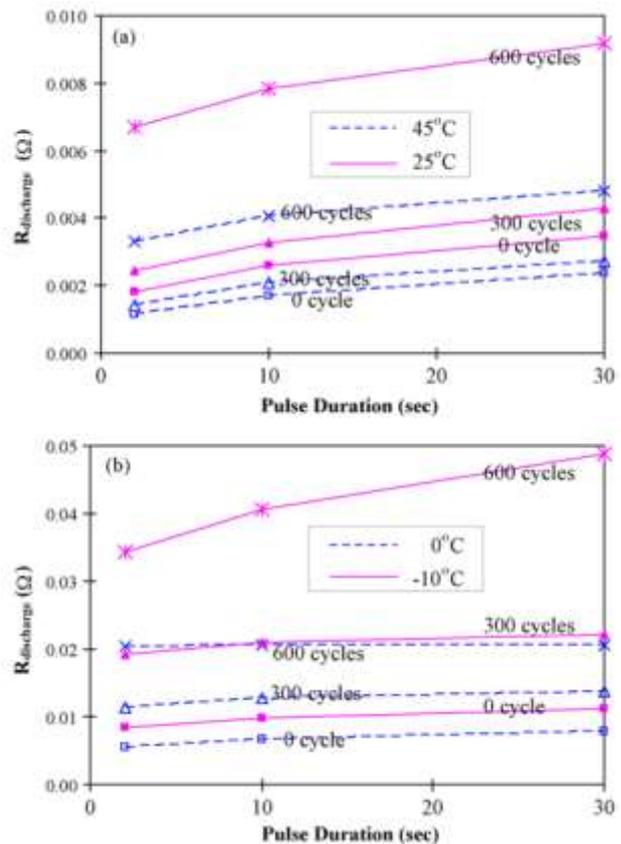
Figure 76. Discharge resistance changes with pulse duration after different cycles (a) at 45 and 25°C, and (b) at 0 and -10°C.
