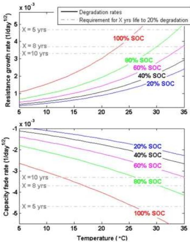
Figure 51. Typical graphite/NCA degradation rates for storage at constant SOC and temperature (solid lines). Dotted lines show maximum allowable degradation rates for example end-of-life requirements of 20% resistance growth and 20% capacity fade. [69]
