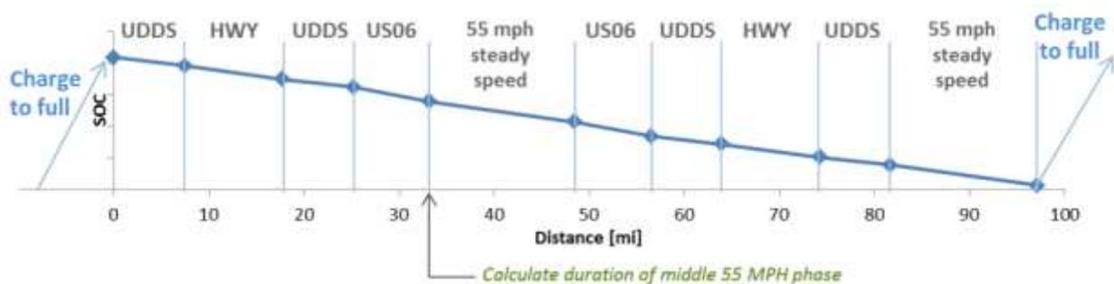
Figure 92. Multi-Cycle Test for BEV used by Argonne National Laboratory (Simplified) [87]
