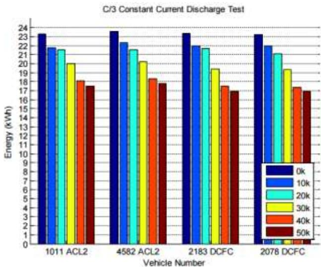
Figure 33. Battery capacity discharged for each pack at 10,000 mile intervals. Each result is the average of three 3-hour constant current discharge tests, falling within 2% of each other. [62]
