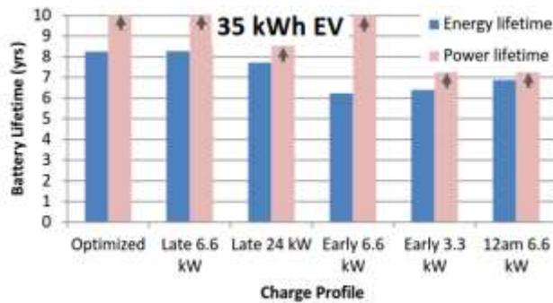
Figure 87. 35 kWh battery lifetime under various charge scenarios. Power lifetimes truncated. [85]
