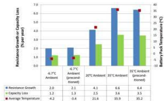
Figure 59. PHEV15 battery degradation rates (left axis) and average temperature (right axis) [72]
