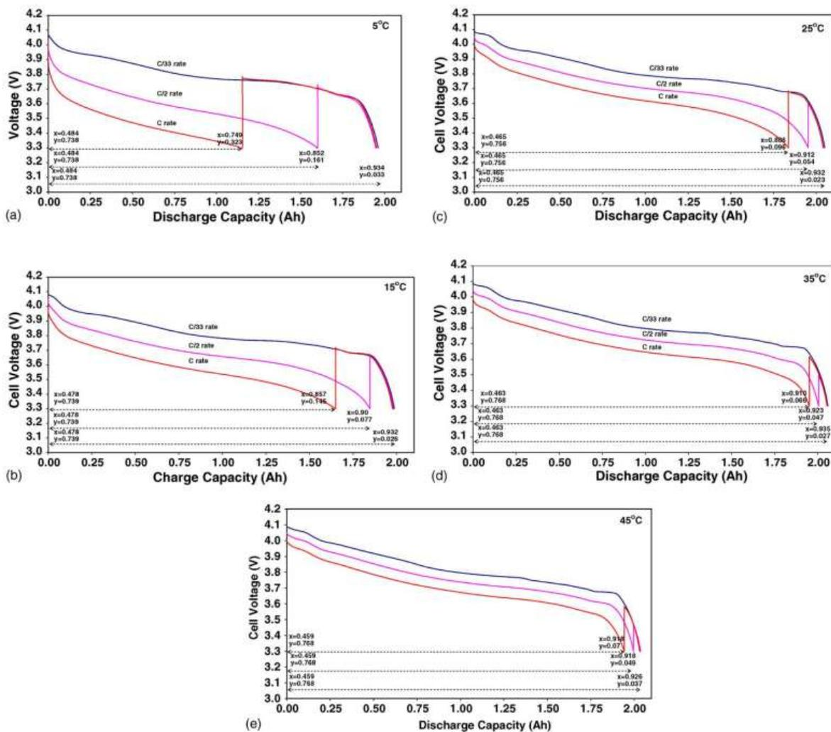
Figure 17. Rate capability at various temperatures. The vertical lines of curves at the end of C/2 and C rates correspond to the 30 min relaxation period. The states of charge of anode (y in  $\text{Li}_y\text{C}_6$ ) and cathode (x in  $\text{Li}_x\text{CoO}_2$ ) are given at the beginning and end of discharge at each rate. (a) 5 °C, (b) 15°C, (c) 25°C, (d) 35°C and (e) 45°C. [21]
