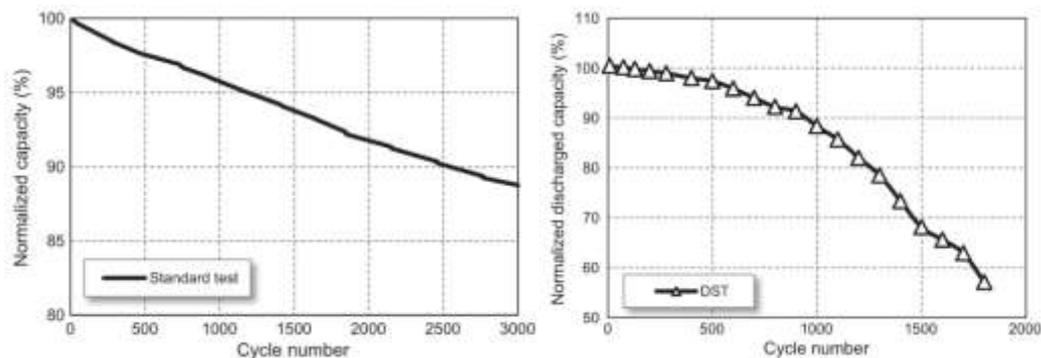
**Figure 77. Cell 1 from [5] subjected to standard tests and USABC DST tests**
