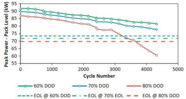
Figure 81. Power degradation at various levels of capacity based DOD as a function of cycle number (fig6) [83]
