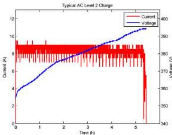
Figure 31. An AC level two charge is shown for a 2012 Nissan Leaf with a 3.3 kW onboard charger [62]
