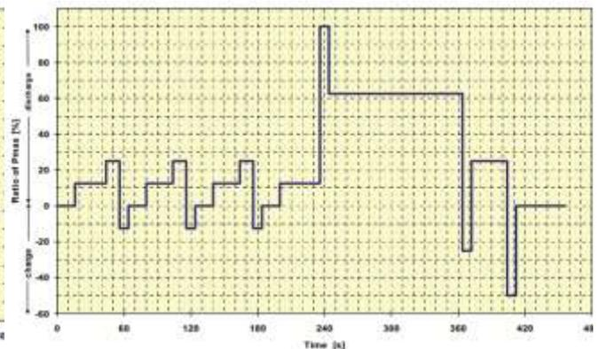
Figure 105. ISO 12405-2 Profile for cycle life test — Dynamic discharge power profile B [102]
