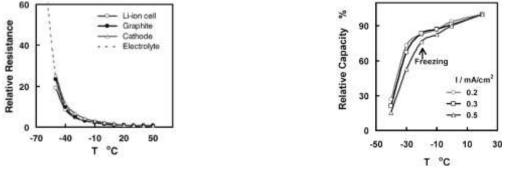
Figure 14. Li-Ion Battery Resistance Increases with Decreasing Temperature [**39**]
