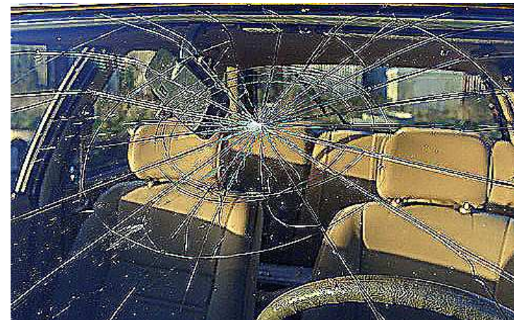
<The fracture characteristic between toughened glass and laminated glass>
