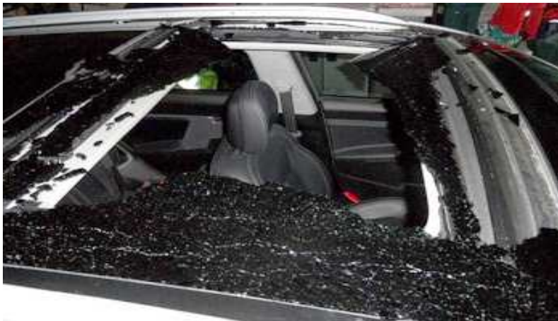
<The fracture characteristic between toughened glass and laminated glass>
