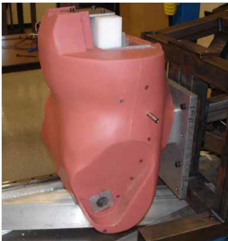
Figure 2-5: BioRID jacket certification set-up
