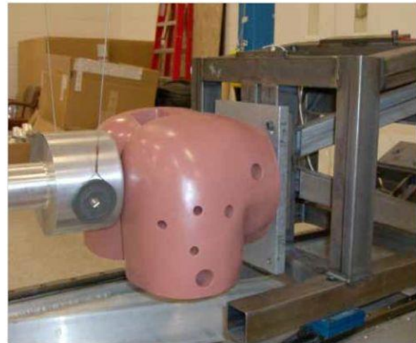
Figure 2-6: BioRID pelvis certification set-up: rear impact left; base impact right
