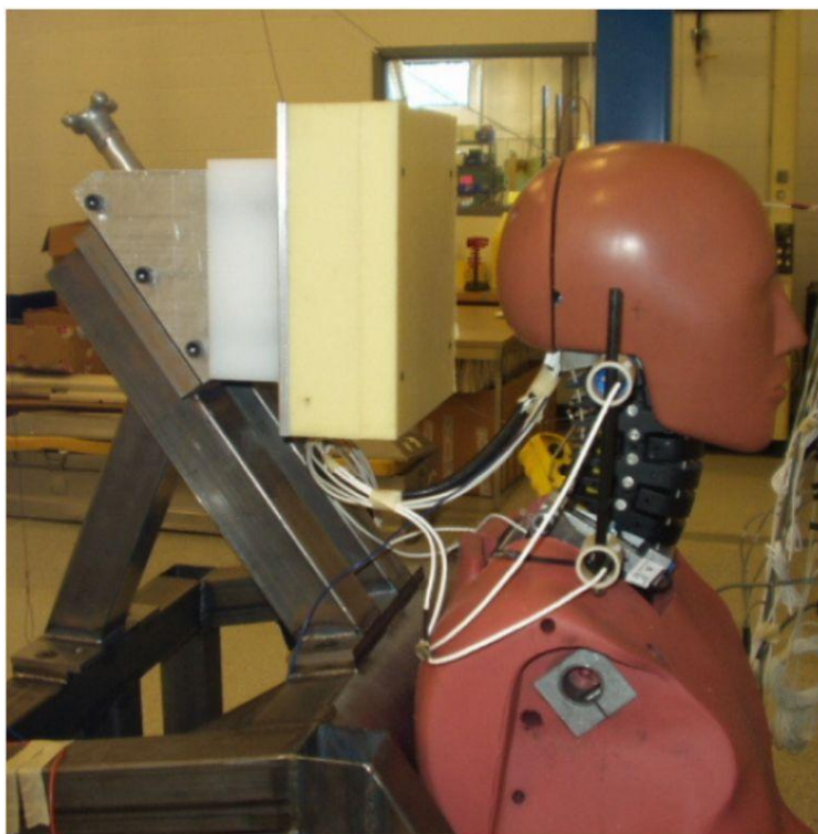
Figure 2-4: BioRID with head restraint certification set-up
