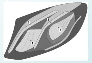
1 Fibre-optic LEDs
