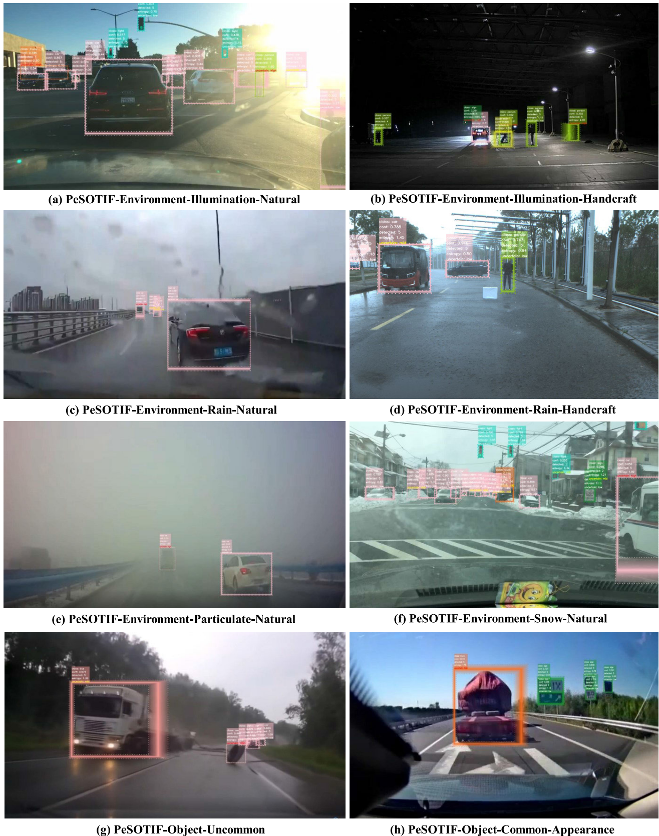
Fig. 10. Perception results with entropy in key frames of some typical SOTIF scenarios in the PeSOTIF dataset. Objects with low, medium, and high entropy are labeled white, yellow, and red on the last line of the box information, respectively.
