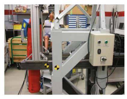
FlexPLI suspension frame mounted on test stand
