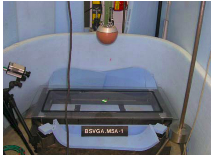
Photo 5: Adult headform drop test – impact point
