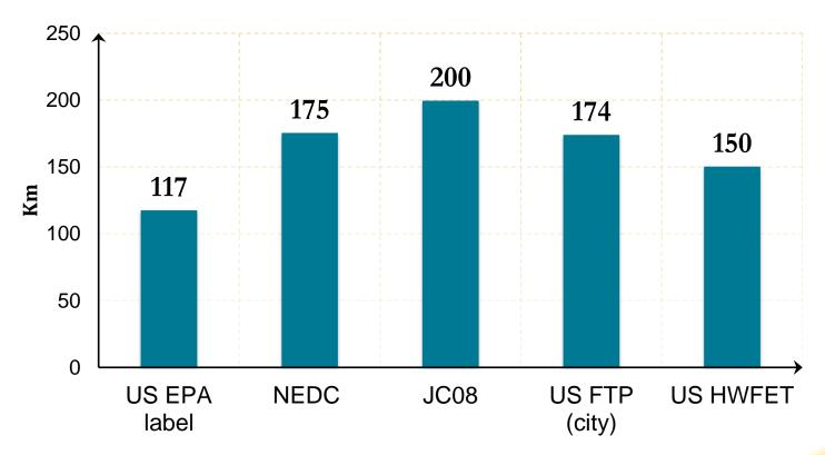
US EPA consumer label estimate and global test cycle measurements of Nissan Leaf range (sources: Nissan, US EPA)
