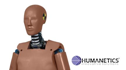
• The new corridors have functioned with relatively consistent accuracy, with the *exception of the first portion of POT A rotation*, which is a forward rotation of the head about the occipital condyle pin.
