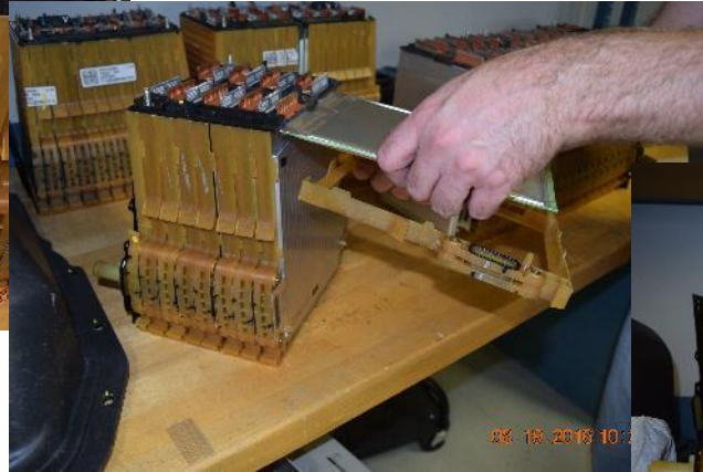
Remove holding frame to fit heater
