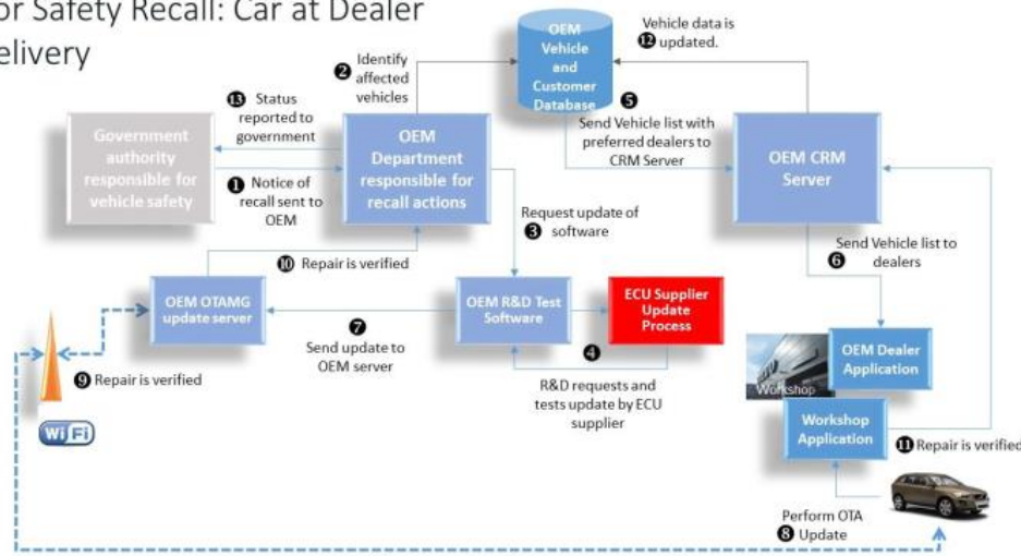
Figure 13: Potential process for an OTA firmware update for a safety recall for car pre-delivery at dealer (Sena Consulting, 2016).
