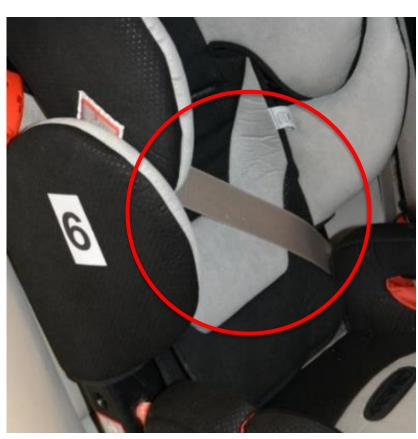
Belt should be routed underneath the back rest cushion
