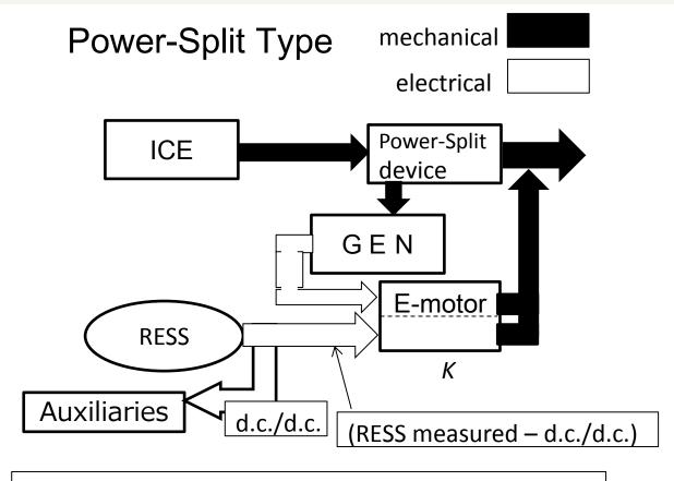
Part of RESS converted to mechanical power by motor (RESS measured – d.c./d.c.) x K
