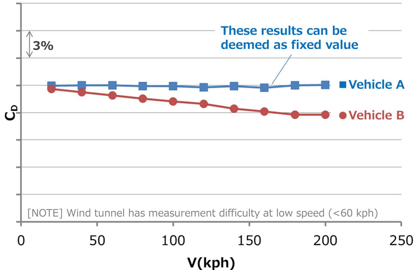
**Vehicle without movable aero parts might also have aerodynamic drag depending on “speed”**
