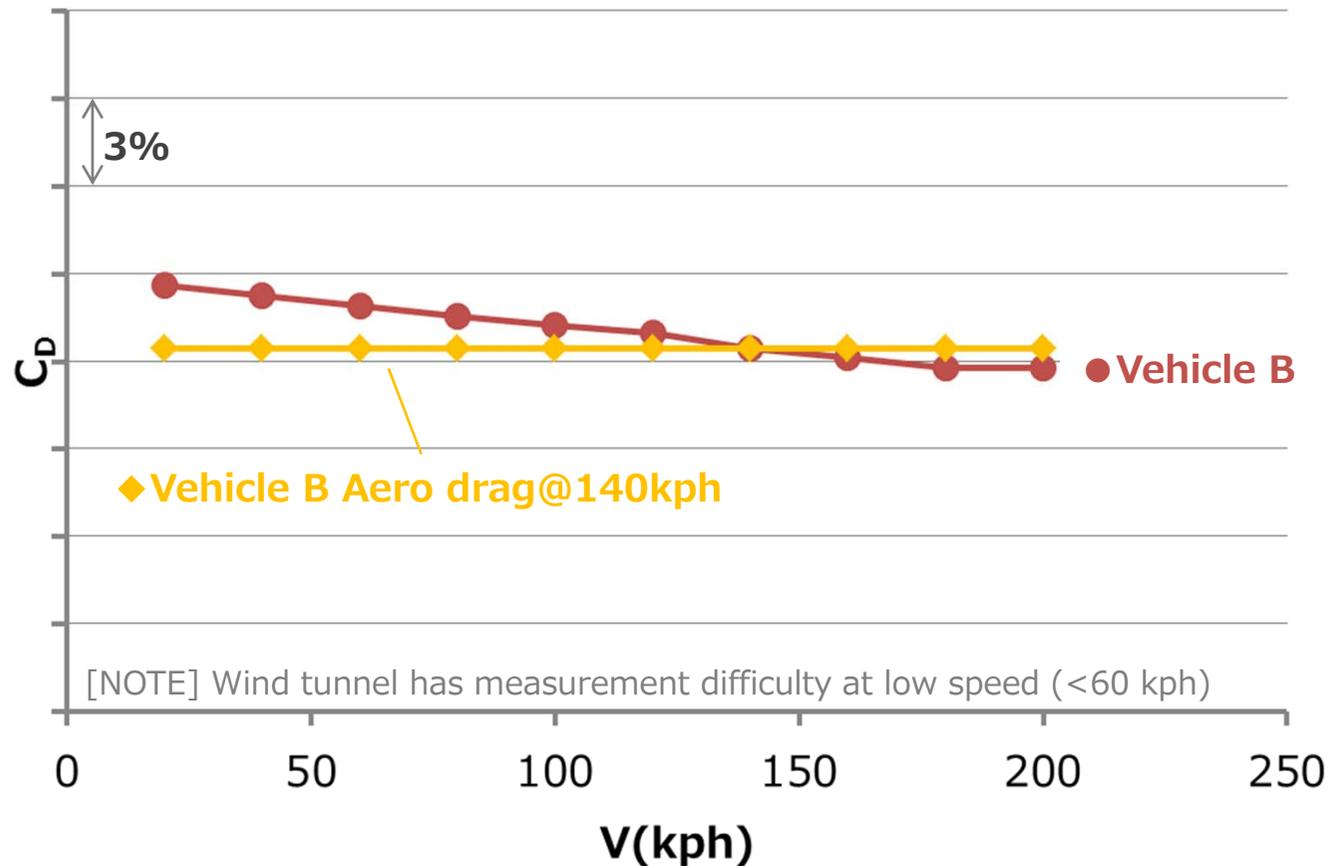
For vehicle B, MAX 3% difference cause at low speed.
