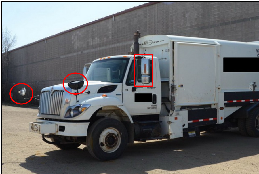
Figure 2: Mirror Installation on a Recycling Truck
