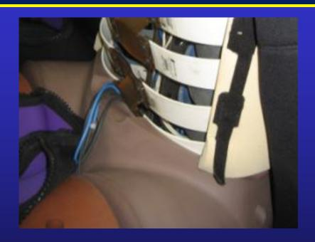
Testing has confirmed that this interference has negligible effects and the ISO WorldSID Task Group has recommended no changes to the dummy design.
