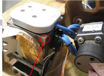
After modifying the pelvis, VRTC still observed minor contact during pelvis impactor tests conducted at 6 m/s (cert test speed is 6.7 m/s)
