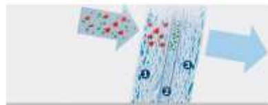
● Dust, pollen and dirt particles ● Particulates, diesel soot and bacteria 1 Preliminary filter 2 Carrier fleece 3 Microfiber fleece
