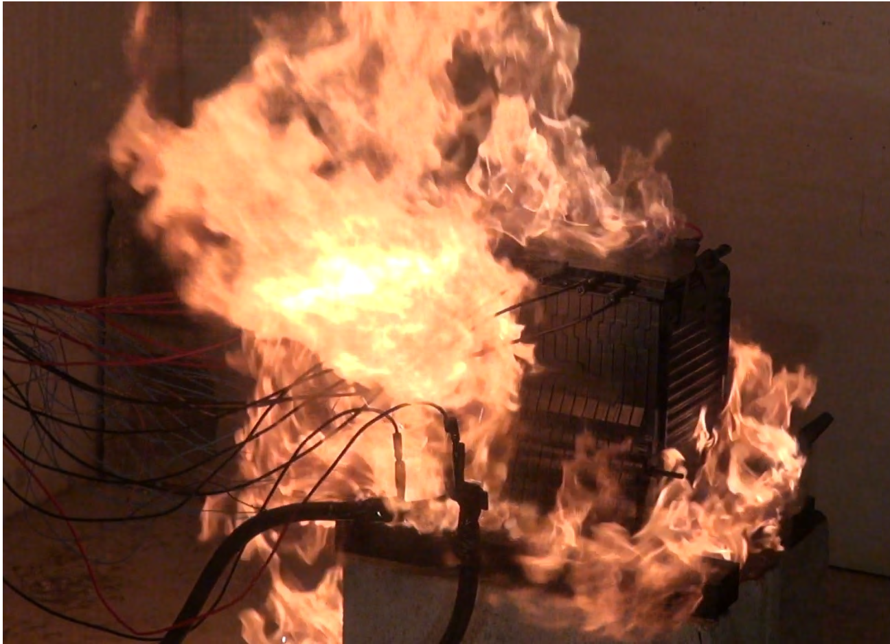
Figure 3. View of module type A taken 10 seconds after failure initiation.
