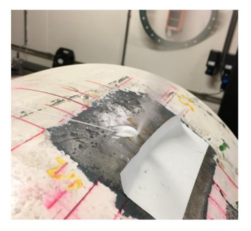
Failure mode: **Hydrogen enhanced fatigue** for metallic vessel and metal liner of composite cylinders
