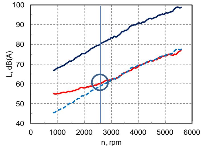
$L_{pt, NL} = 59.3 \text{ dB @ } 2620 \text{ rpm}$
