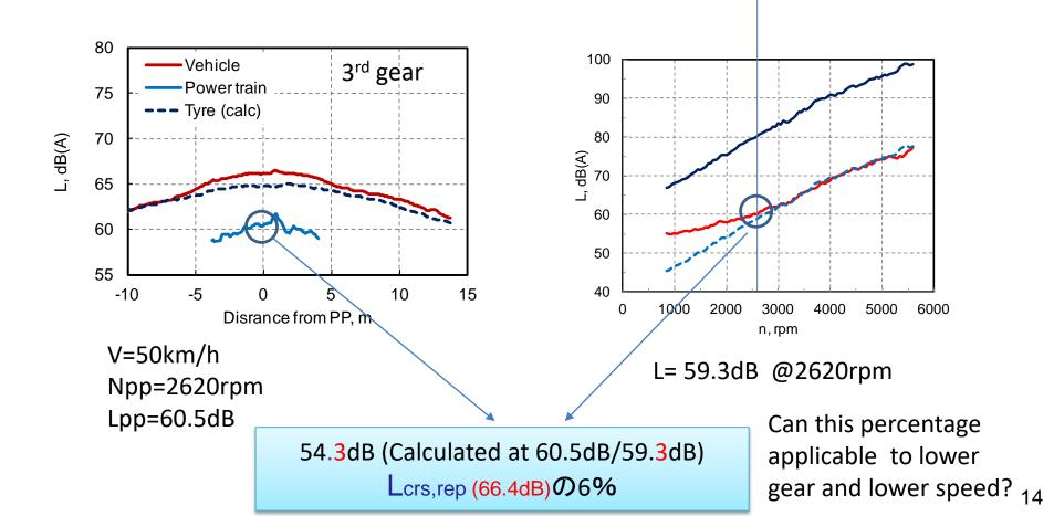
1 The "Prediction Model" for the **Tyre Rolling Sound** LTR,NL = Slopetr \* LOG10(Vtest / 50) + LREF,TR
