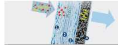
● Dust, pollen and dirt particles ● Particulates, diesel soot and bacteria ● Harmful and odorous gases 1 Preliminary filter 2 Carrier fleece 3 Microfiber fleece 4 Activated carbon
