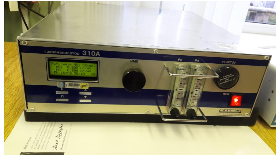
Gas analyzer "R-310A" with chemiluminescent detector for determination of nitrogen oxides NO, NO 2
