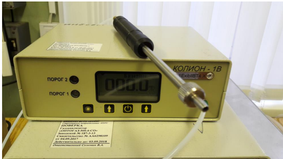
Gas analyzer "Kolion 1B" with photo-ionization detector for determination of aromatic hydrocarbons in terms of benzene
