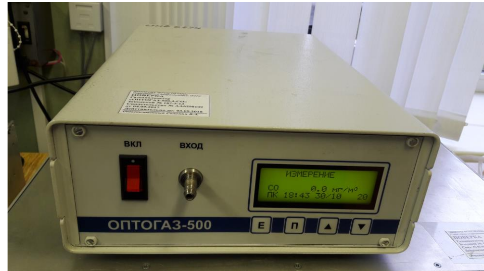
Gas analyzer "Optogas 500.4-CO" with electro-chemical detector for determination of carbon monoxide, CO
