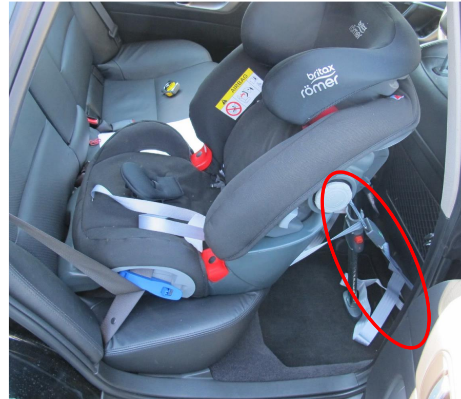
Figure 3 – Installation of a RWF CRS using lower tethers
