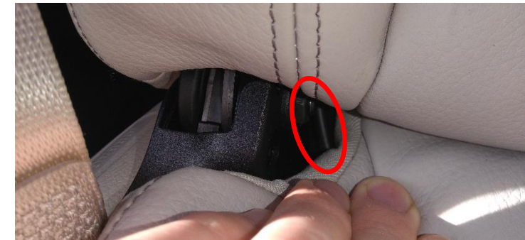
Figure 5 – Example for wire routing at a front vehicle seat
