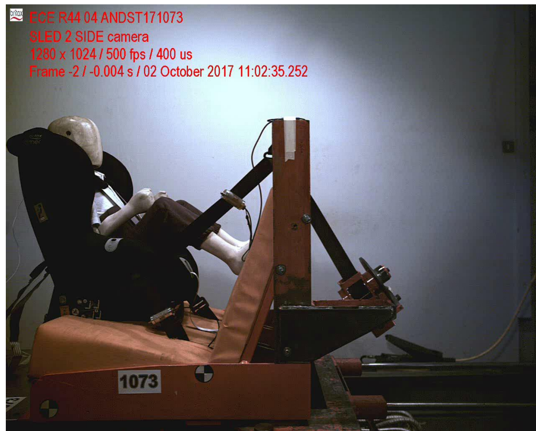
Video 1 – Example of a rear impact test according to R44 with a RWF CRS using LT's
