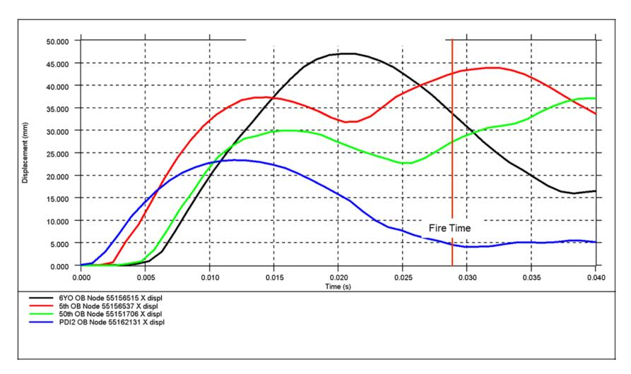
Significantly less displacement into a vehicle fascia by PDI-2
