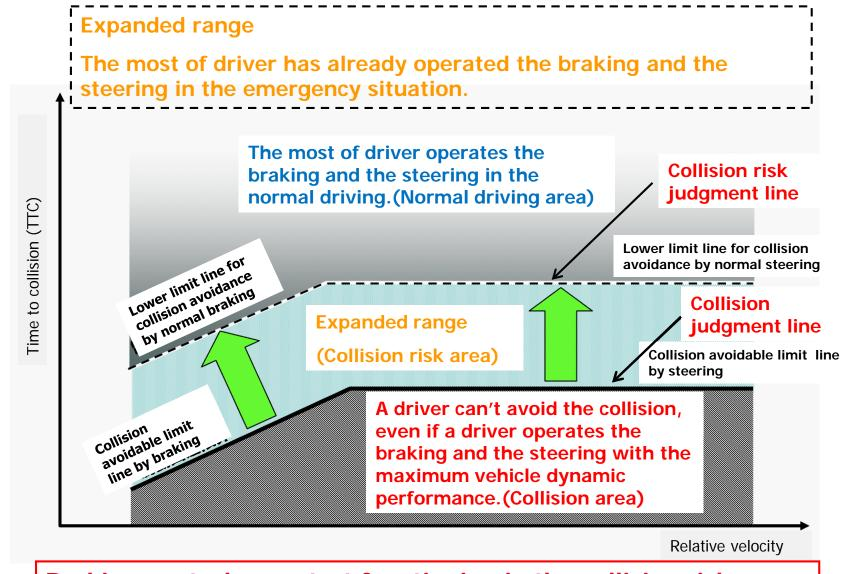
Braking control may start functioning in the collision risk area.
