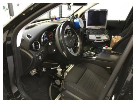
Task: Robot programmed for lane change maneuver 0.9/1.0/1.1 s Lane change width: 2m Robot peak torque: 15 Nm (ABD SR15+CBAR Robot System)
