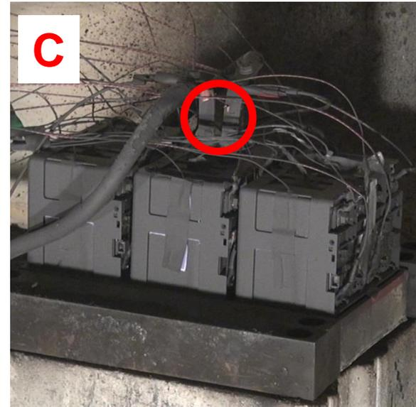
Three extracted xEV battery modules under test (types A, B and C).
