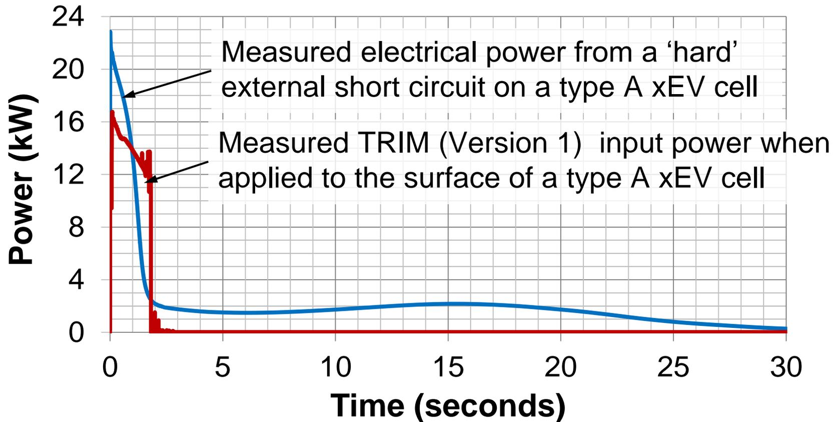
Comparison of TRIM input power applied to a type A xEV cell to the measured power during a 2.2m $\Omega$  external short circuit on an identical cell.
