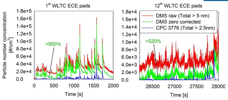
DMS500 overestimation was evident at all concentration levels and could not be related to background levels that were also varying → Importance of transparent inversion algorithms and calibration.
