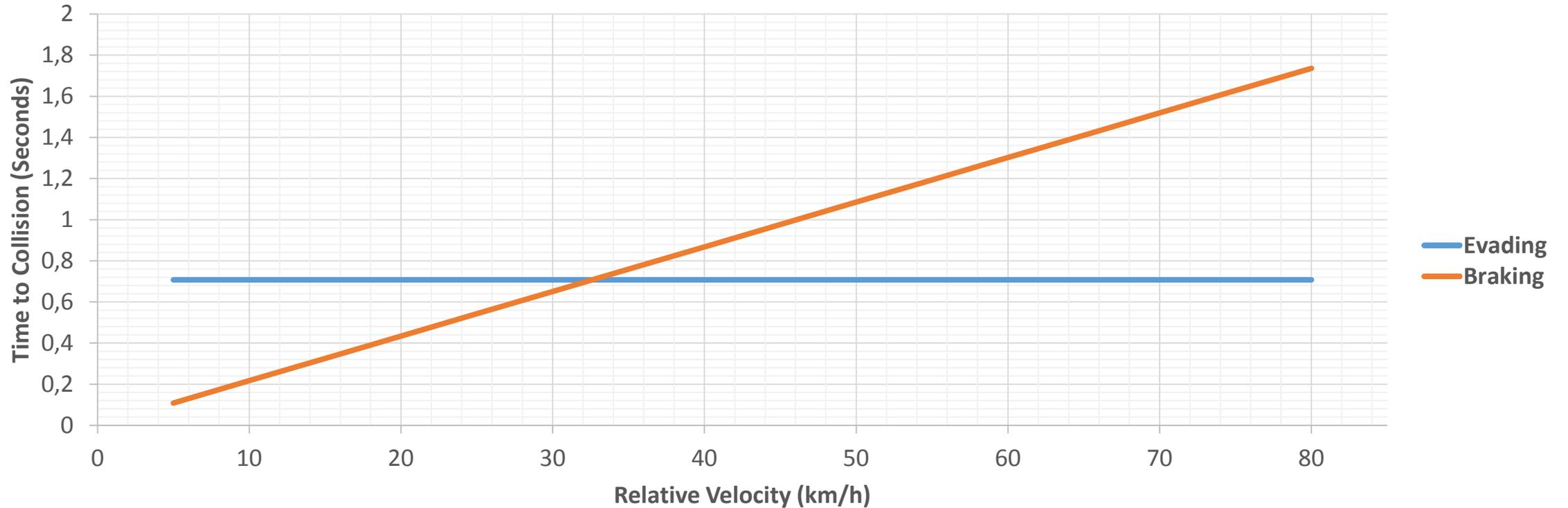
Assumptions: *Braking Level = 6.4 m/s<sup>2</sup> Lateral Acceleration = 10 m/s<sup>2</sup> Lateral Offset = 2.5m*
