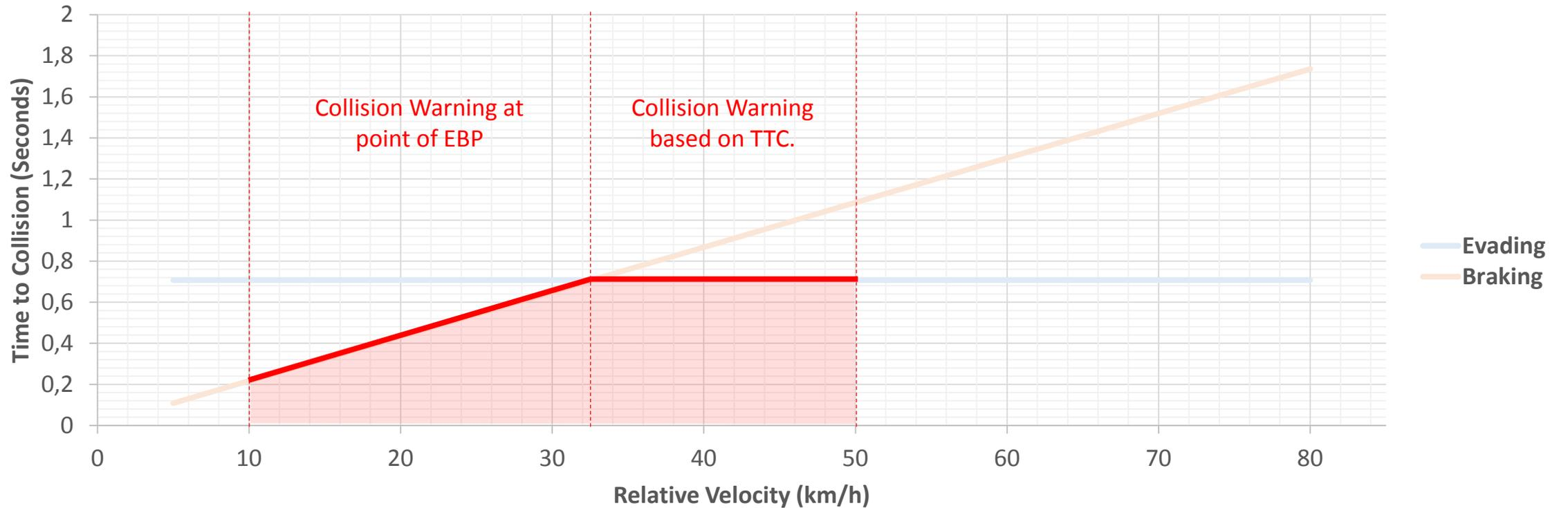
3. The collision warning phase shall activate before the Emergency braking phase, this is only applicable at speeds higher than [32.6]km/h (LPS = LPB), below this speed the Collision Warning shall occur at the same time as the Emergency braking phase.
