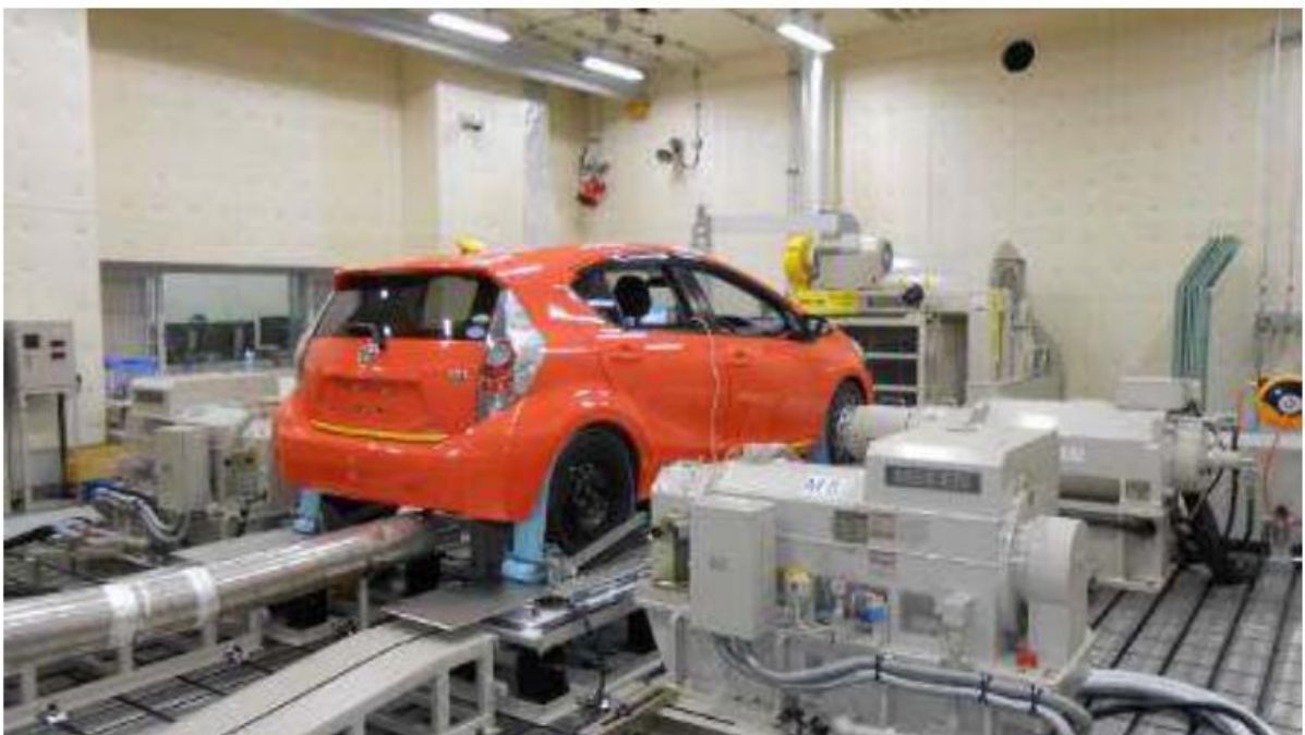
Figure 5.3 Axle-hub chassis dynamometer test (testing vehicle A)
