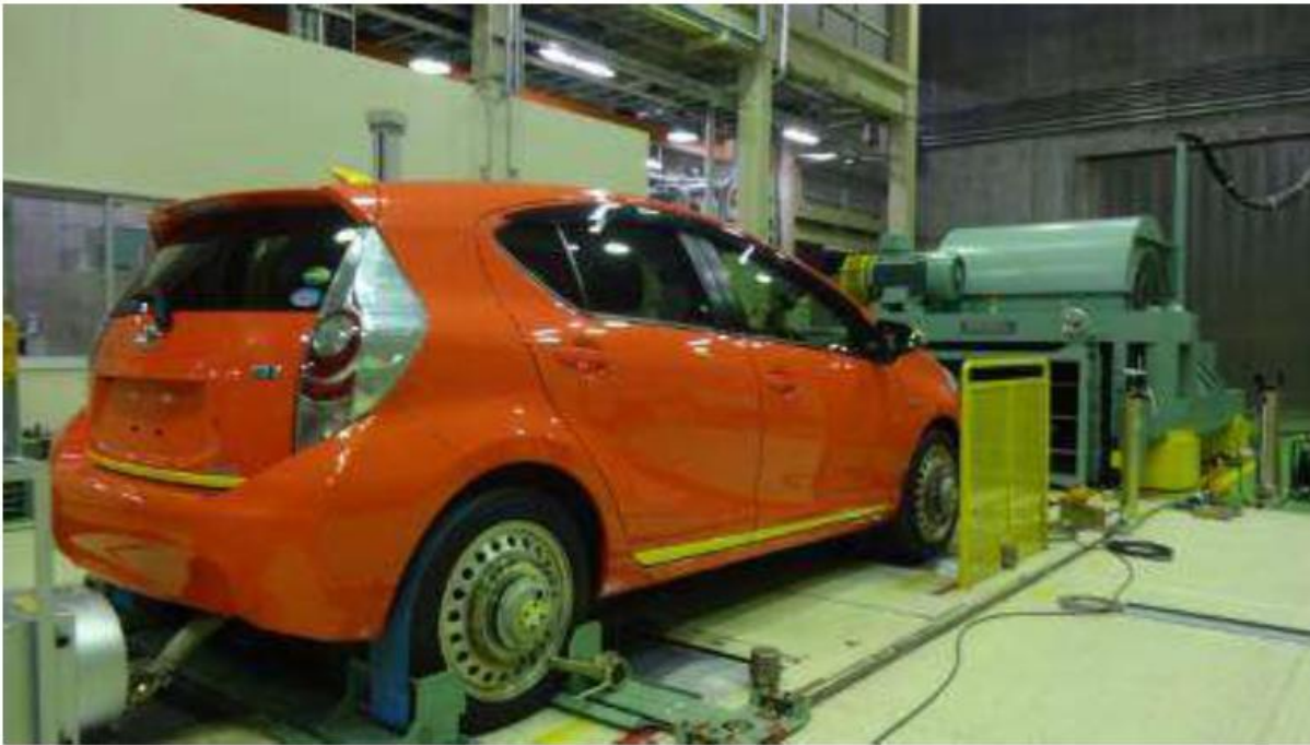
Figure 5.2 Chassis dynamometer test (testing vehicle A)
