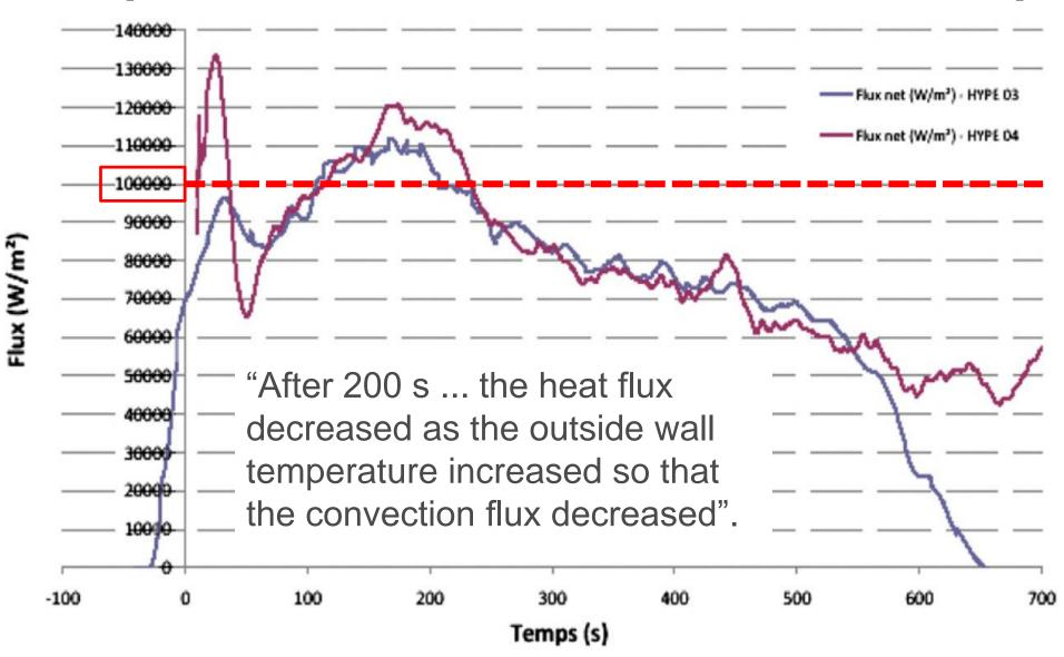
Source: S. Ruban et al., 'Fire risk on high-pressure full composite cylinders for automotive applications', IJHE, 2012.
