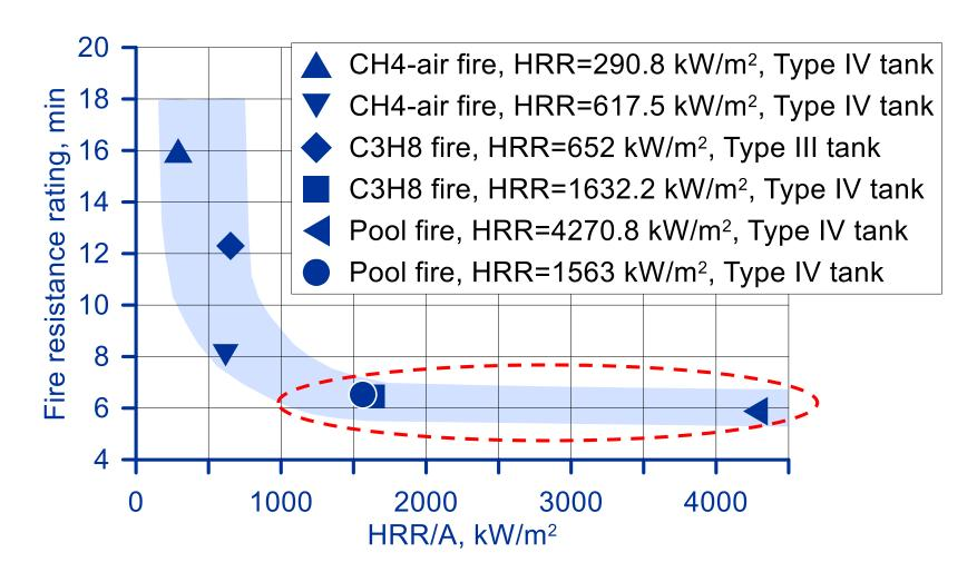
Specific HRR saturation at about HRR/A>1000 kW/m<sup>2</sup>
