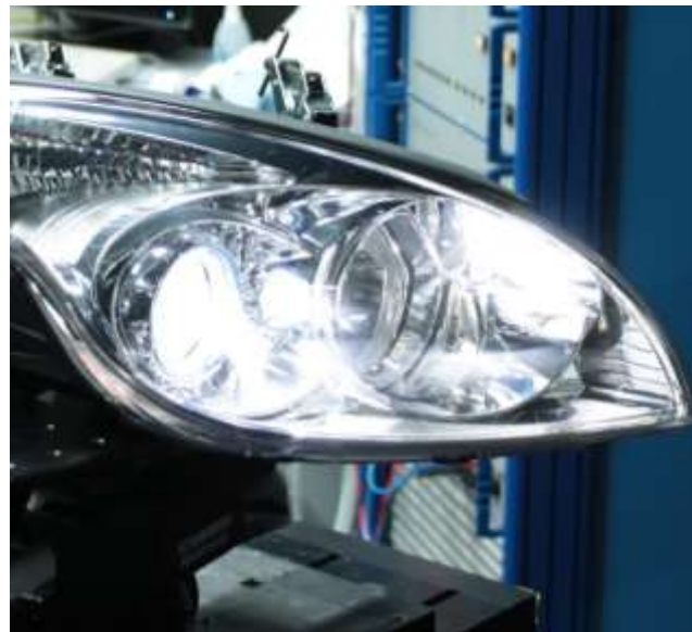
Osram H7 LED Retrofit lamp in Hyundai i30 head light
