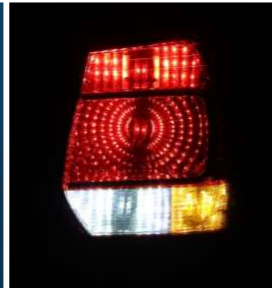
Philips LED Retrofit lamps in VW Golf VI Variant rear light with clear cover
