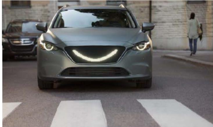
> LED fields in the front show, if the car is driving autonomously (blue) or is controlled manually (white)
