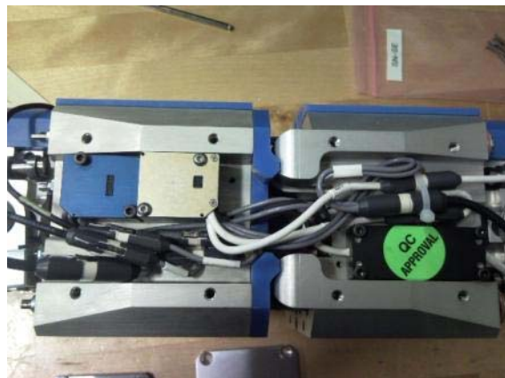
Figure 37 . Left side wiring example of 24 channel SLICE
