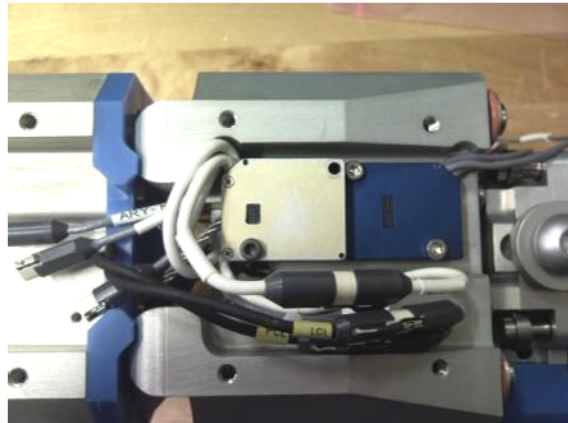
Figure 36 . Optional SLICE unit 24 channel option (right side)
