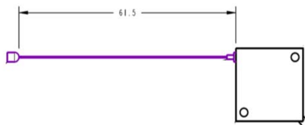
Figure 70 . String potentiometer pull wire length \pm 1mm
