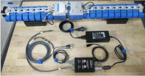
Figure 35 . Leg with disconnect wire, TDAS interface and power supply
