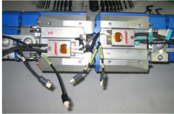
Figure 25 . Right hand side of knee M=BUS 24 channels, sensors not connected
