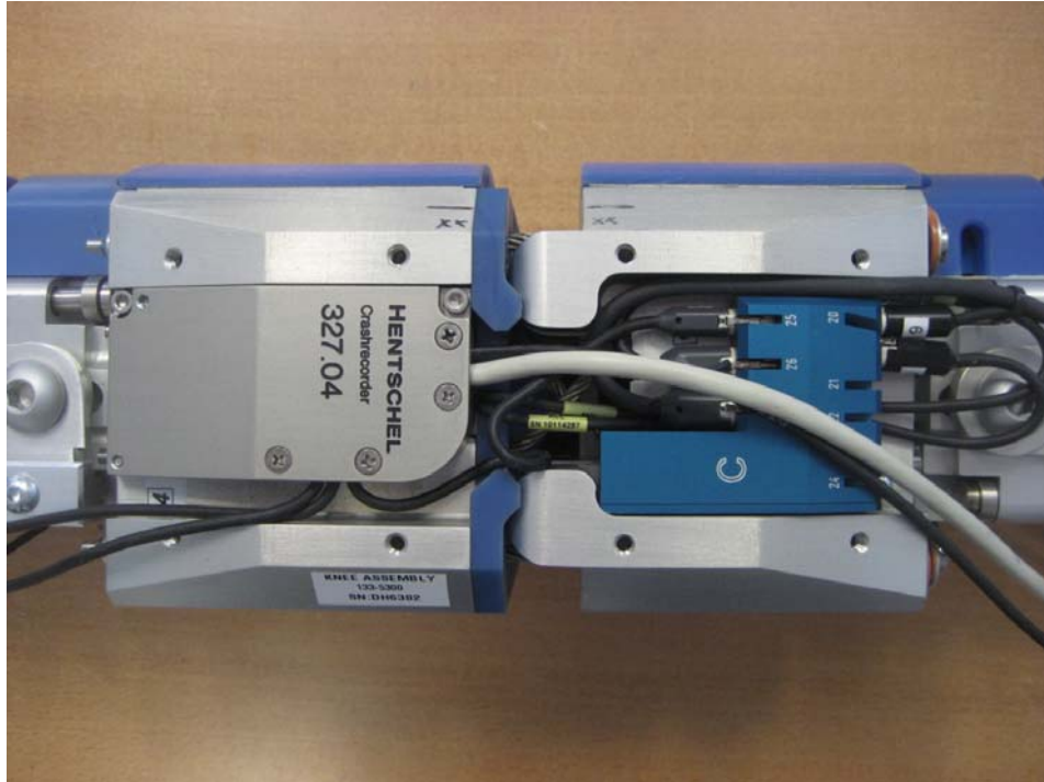
Figure 39 . DTI DAS right hand side of knee showing crash recorder on the left and DiMod hub on the right.
