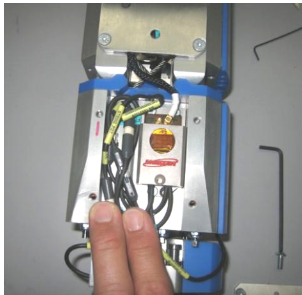
Figure 27 . Bottom right hand side of knee M=BUS 24 channels, sensors connected
