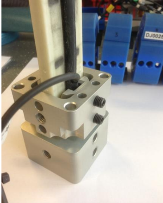
Figure 49 . 133-8129 base with 133-5514 segment, bone clamps and bone assembly
