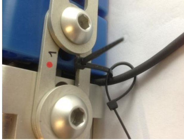
Figure 52 . Bone exit cable restraint use cable ties (ties not shown trimmed or tightened)
