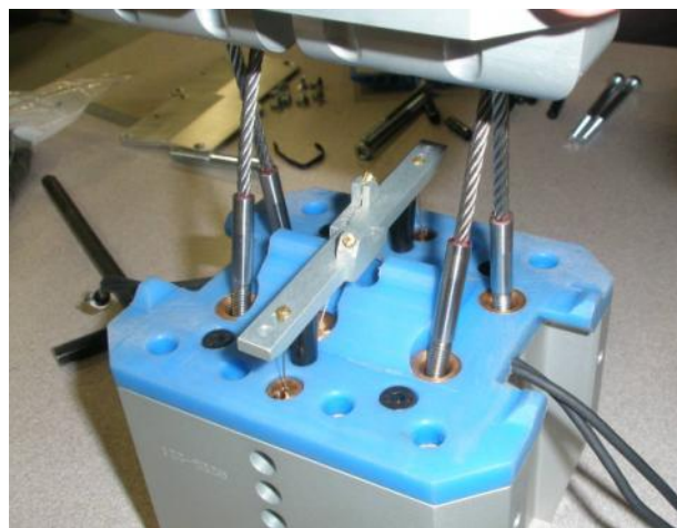
Figure 58 . Cross wire feed through on knee
