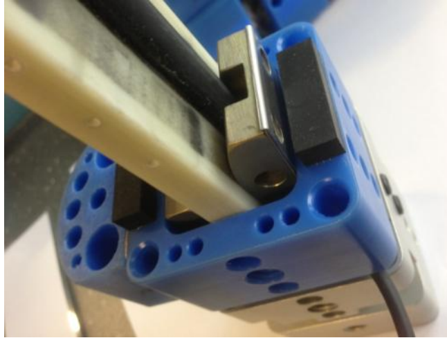
Figure 51 . Fitting thin bone spacer with captive shim
