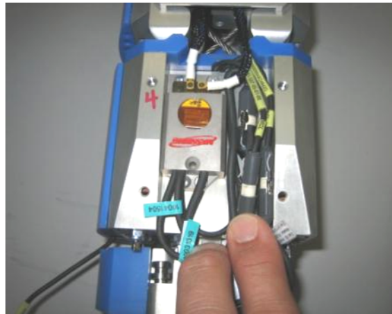
Figure 29 . Bottom left hand side of knee M=BUS 24 channels, sensors connected
