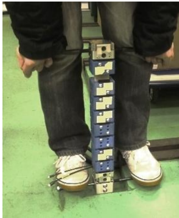
Figure 62 . Fitting last two segments to tibia, applying force using M10 bolts
