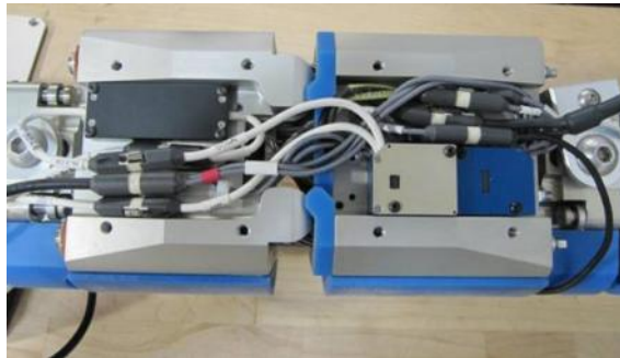
Figure 31 . Typical 12 channel Slice wiring to knee
