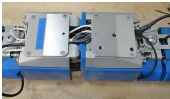
Figure 33 . LH of leg with knee covers fitted 12 channels. Leg wires are not shown secured.
