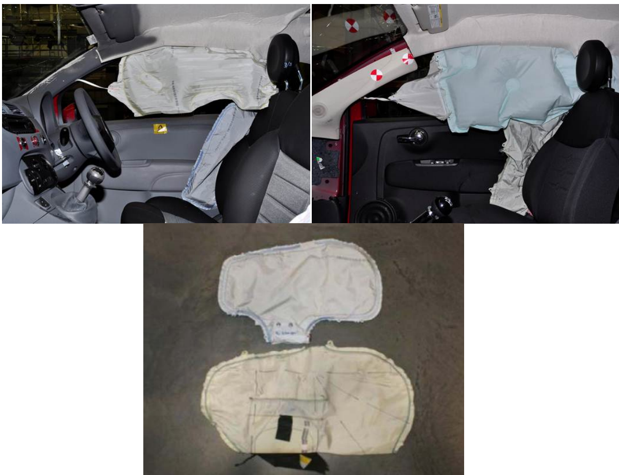
Figure 8.2 Comparison of curtain and thorax side airbags (below) fitted to the same vehicle model in the Australian and North American market (supplied by T. Belcher)
