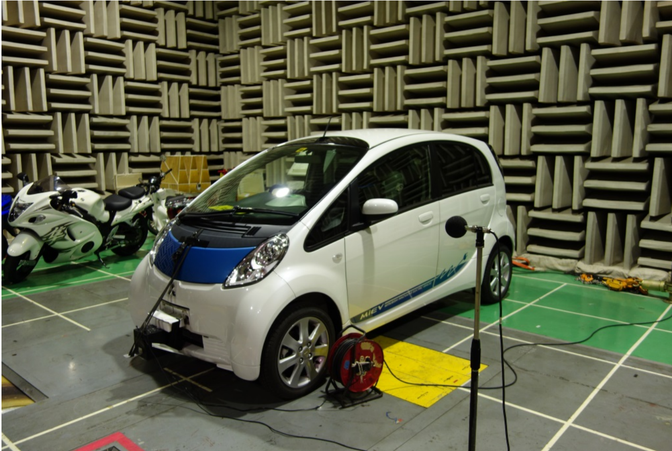
Speaker attached to the tip of EV
