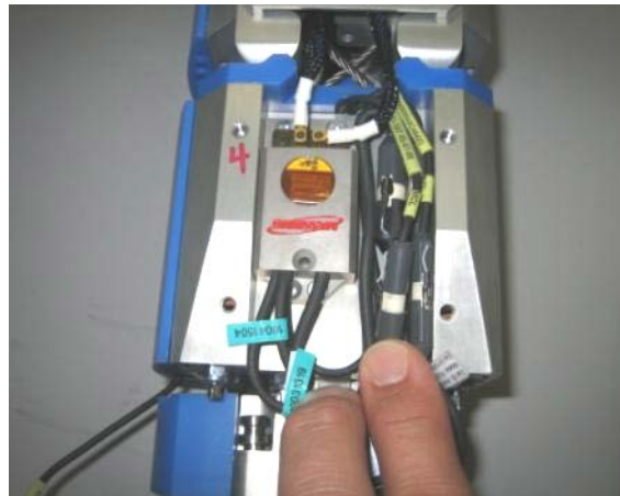
Figure 30 . Bottom left hand side of knee M=BUS 24 channels, sensors connected
