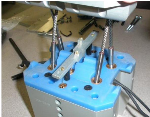
Figure 65 . Cross wire feed through on knee
