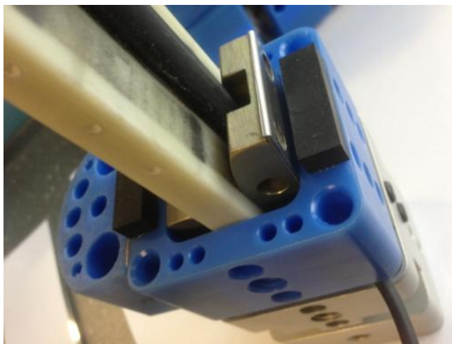
Figure 58 . Fitting thin bone spacer with captive shim
