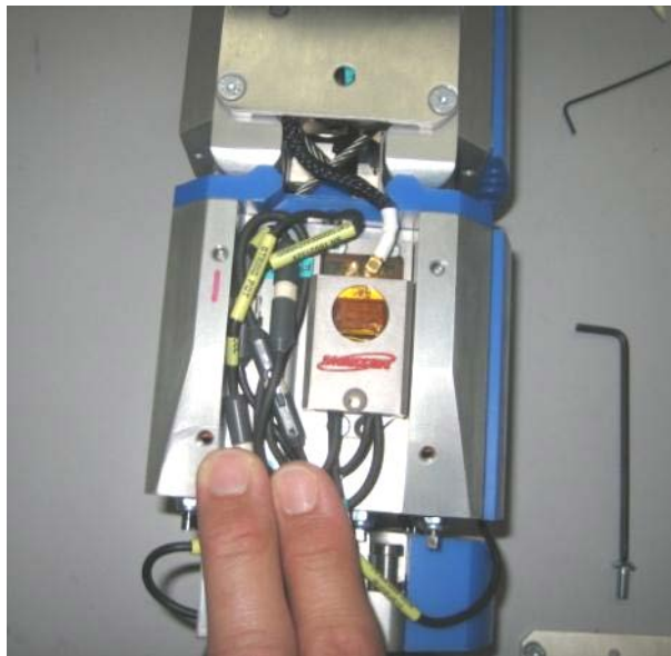
Figure 28 . Bottom right hand side of knee M=BUS 24 channels, sensors connected
