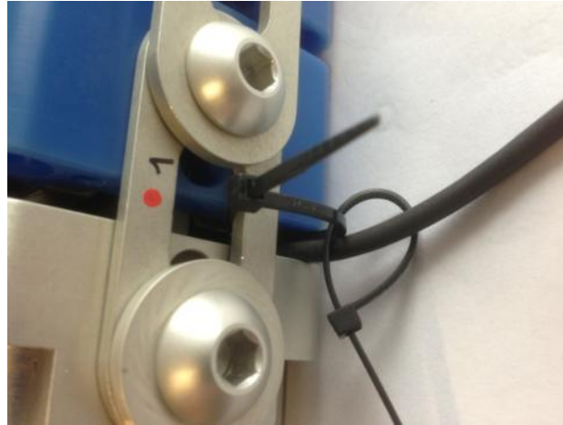
Figure 59 . Bone exit cable restraint use cable ties (ties not shown trimmed or tightened)
