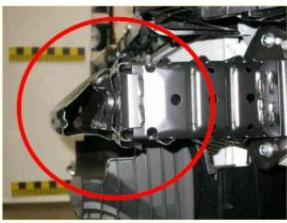
Stiff structures beneath the front bumper panel and outboard of the bumper bar and pedestrian protection structures were associated with the poor performance.
