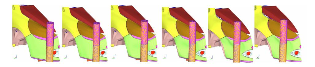
The EEVC legform turns outwards, with few severity observed on the criteria.
