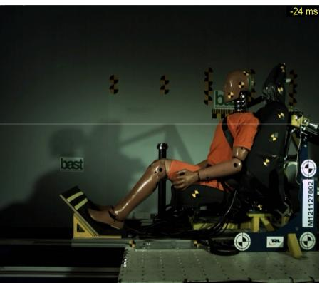
Acceleration sled, TRL/EC lab seat, draft GTR 7 Annex 9 pulse (JNCAP style)
