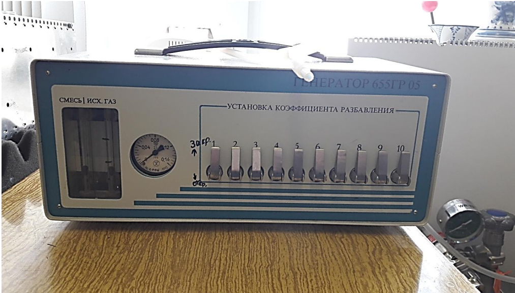
Dynamic divider (gas mixture generator) mod.655 GR05
