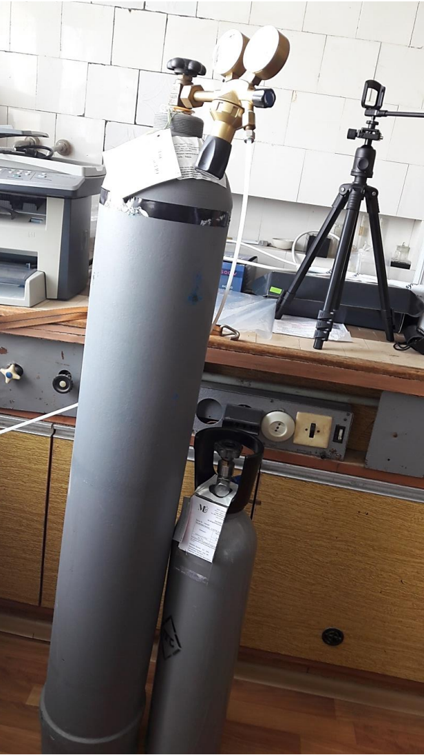
The gas cylinder with working gas (synthetic air)
