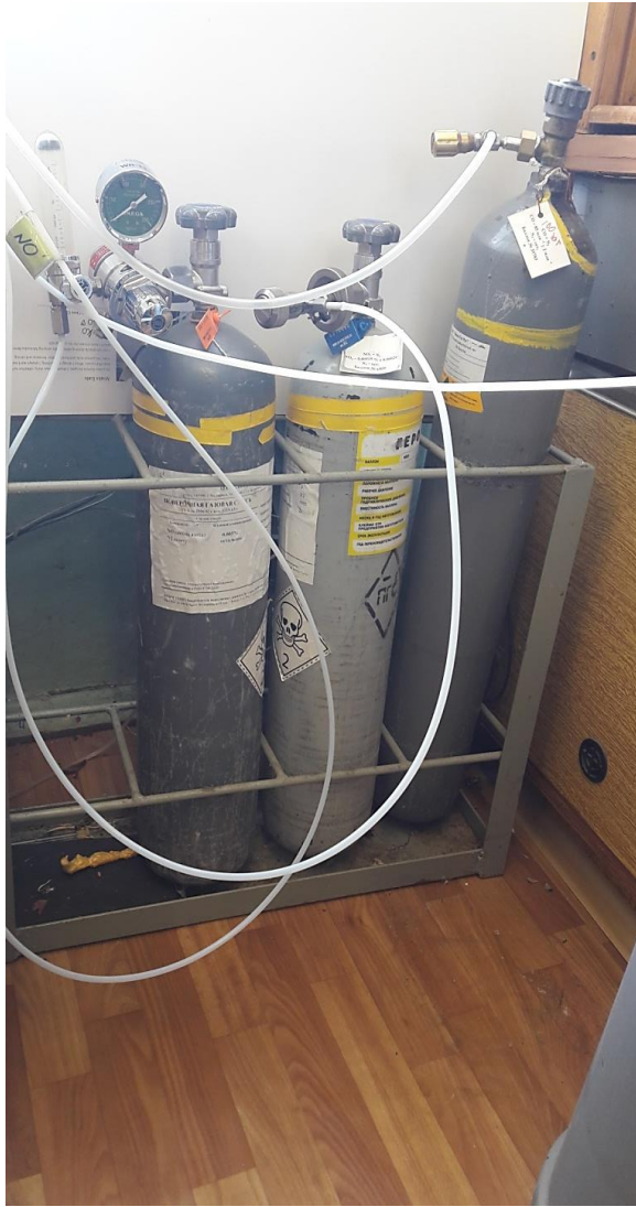
Gas cylinders with calibration gas mixture of calibrated components NO, NO2, CO in nitrogen
