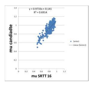
Evident linear relation between μ-cand and μ-SRTT16 (track friction)
