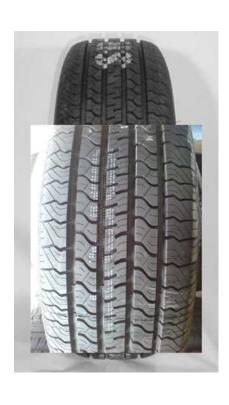
Must be used as **reference tyre** to determine the relative wet grip performance of the candidate tyre
