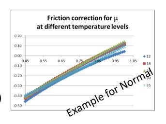
$\mu$ (test) vs track grip  $\mu$ (SRTT16) approximately linear
